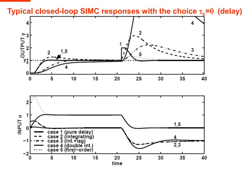
Figure 4: Responses using SIMC settings for the five time delay processes in Table 3 ( $\tau_c = \theta$ ). Unit setpoint change at t = 0; Unit load disturbance at t = 20. Simulations are without derivative action on the setpoint. Parameter values:  $\theta = 1, k = 1, k' = 1, k'' = 1$ .
