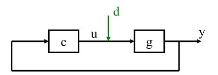
*Example*. "Almost-integrating process" with disturbance at input:  $G(s) = e^{-s}/(30s+1)$ Original integral time  $\tau_1 = 30$  gives poor disturbance response Try reducing it!
