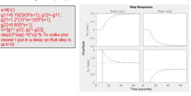
Steady-state gain matrix:  $G(0) = \begin{bmatrix} 0.1925 & -0.1925 \\ 1.2 & 0.8 \end{bmatrix} \Rightarrow$
