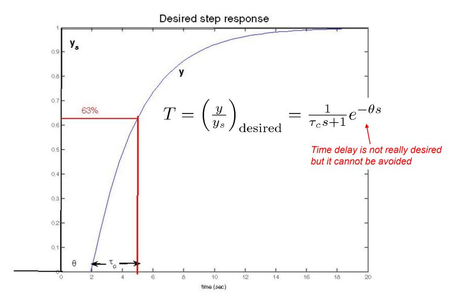
NOTE: Setting the steady-state gain = 1 in T will result in integral action in the controller!
