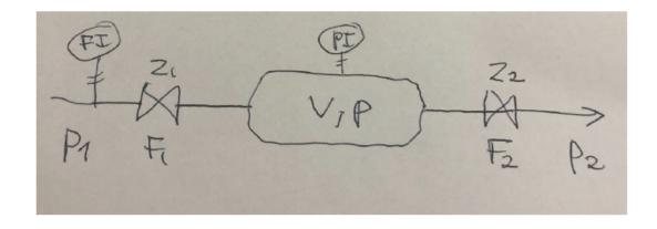
Consider a gas pipeline with two valves. We have measurements of the inflow  $F_1$  and the intermediate pressure p and these should be controlled. The volume of the pipeline can be represented as a tank with volume V as shown in the figure above.
