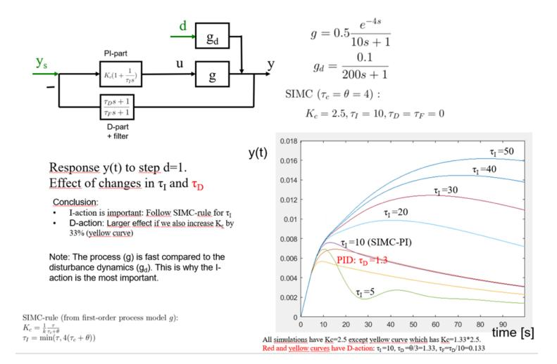
Note: Often D-action requires much more input usage - but in this example the input usage (not shown) is almost the same for all controllers. This is because the disturbance is so «slow» (almost integrating)
