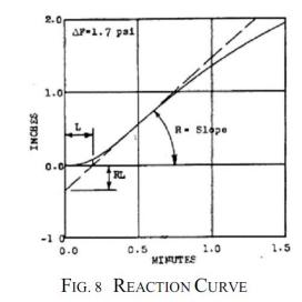
Reset-Rate Determination From Reaction Curve. Since the period of oscillation at the ultimate sensitivity proves to be 4 times the lag. A substitution of 4 L for  $P_u$  in previous equations for optimum reset rate gives an equation expressing this reset rate in terms of lag. For a controller with proportional My notation: reset responses, the optimum settings become Model:  $R = k', L = \theta$
