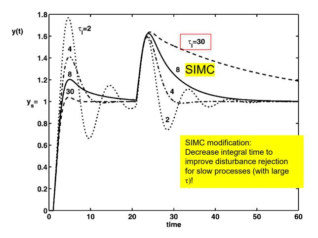
Fig. 3. Effect of changing the integral time  $\tau_{\rm I}$  for PI-control of "almost integrating" process  $g(s) = e^{-s}/(30s + 1)$  with  $K_{\rm c} = 15$ . Unit setpoint change at t=0; load disturbance of magnitude 10 at t=20.
