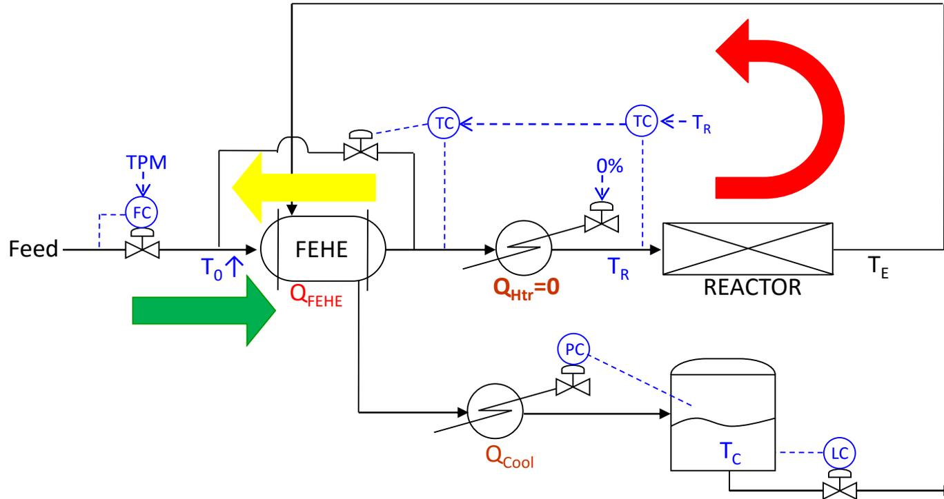
Temperature controller transforms energy balance variability out of recycle loop
