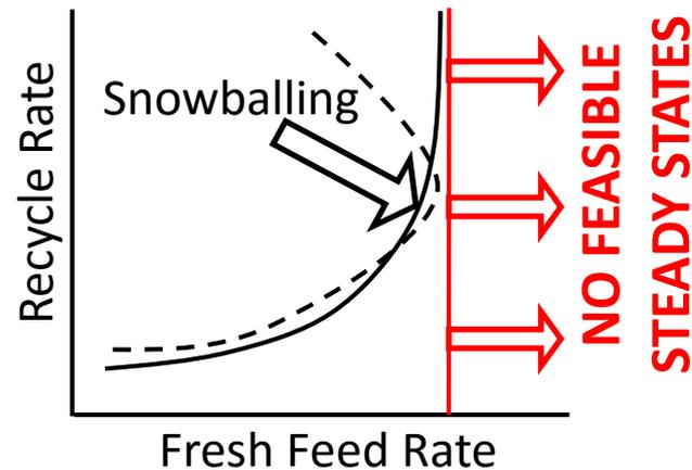
Fixing the fresh feed rate of a recycled component is **NOT** a good idea
