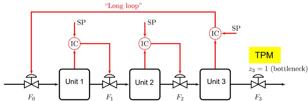
(d) Inventory control with undesired «long loop», not in accordance with the «radiation rule» (for given product flow,  $\text{TPM} = F_3$ )
