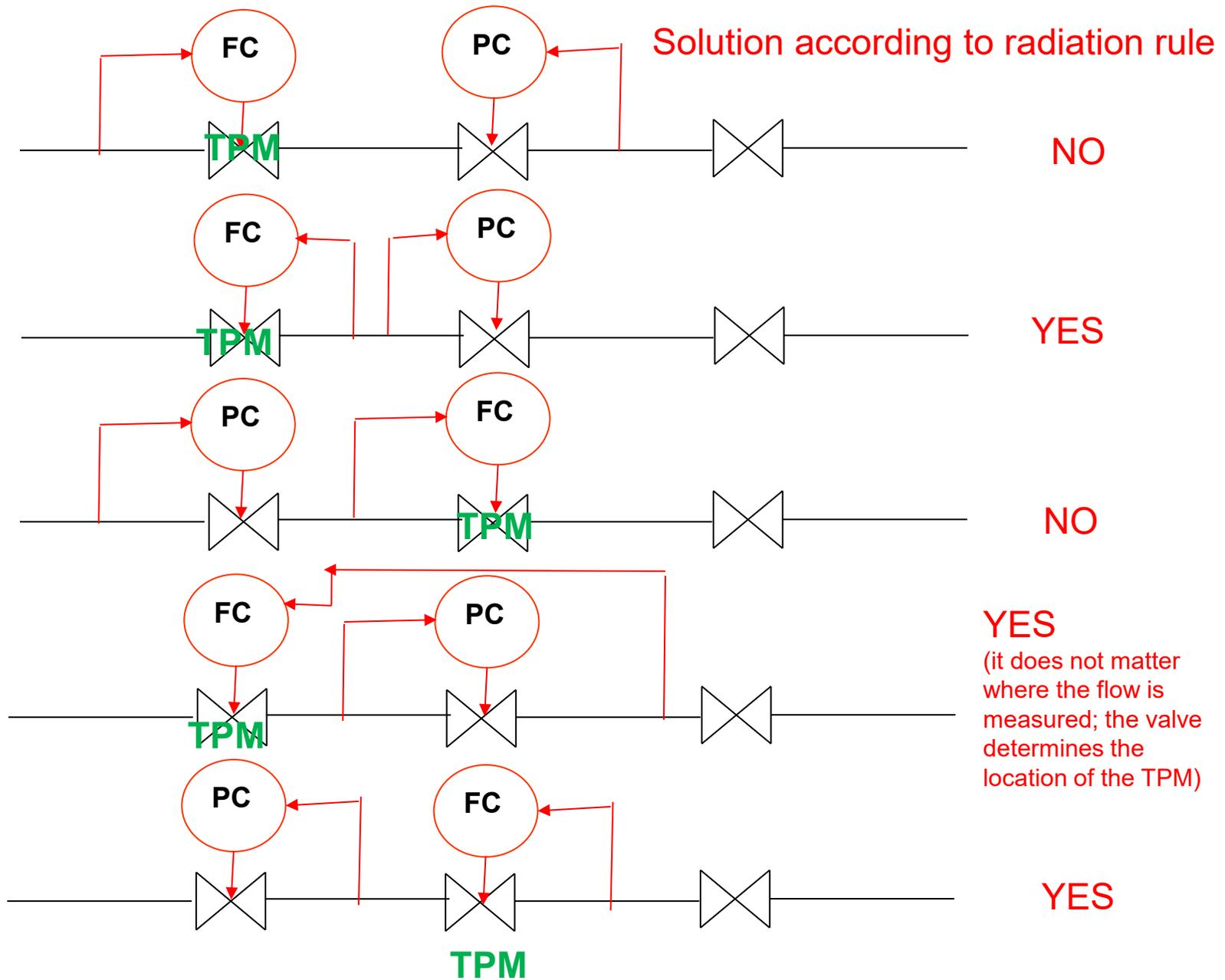
Note: Can never control pressure at ends (upstream first control valve or downstream last valve)!
