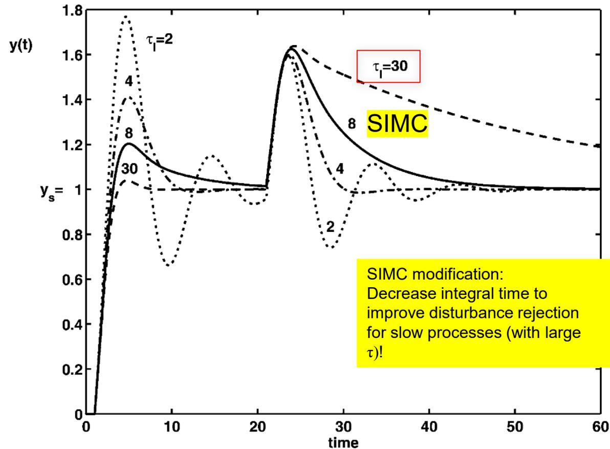
Fig. 3. Effect of changing the integral time  $\tau_I$  for PI-control of “almost integrating” process  $g(s) = e^{-s}/(30s + 1)$  with  $K_c = 15$ . Unit setpoint change at  $t=0$ ; load disturbance of magnitude 10 at  $t=20$ .
