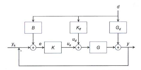
Consider feedforward control with constant setpoint,  $y_s = 0$ . The most common way to implement a combined feedback and feedforward controller is
