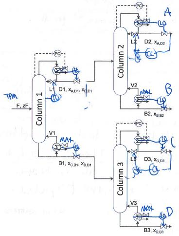
The feed and its composition are given by the upstream processes and our outside of the analysis. The pressure in each column is controlled by the coolant flowrate (see figure).
