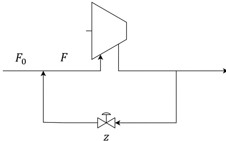
In this system, the compressor must be fed a minimum flow  $F \geq F_{min}$  in order to avoid abnormal operation. However, the system should also operate with the recycle valve fully closed whenever possible, in order to avoid additional compression costs. The process feed  $F_0$  is the main disturbance for the process, and the recycle valve  $z$  is the only available MV.
