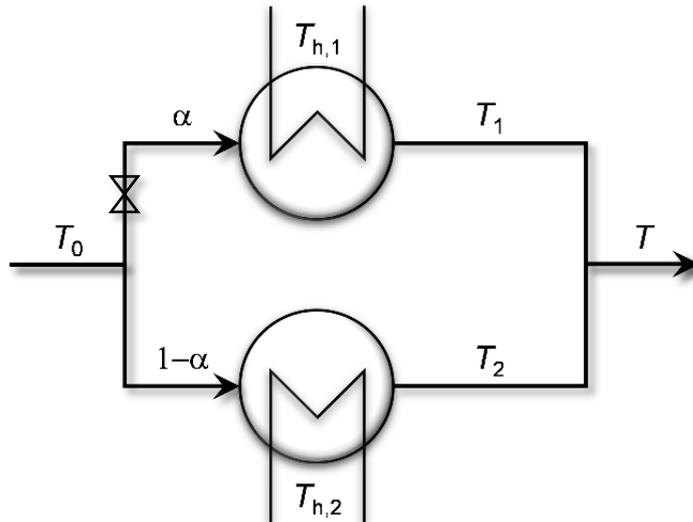
The objective of the operation is to maximize the outlet temperature ( $J = T$ ). In Exercise 1 we derived a simple analytical expression for the cost gradient,  $J_u = \frac{1}{2} \left( \frac{(T_2 - T_0)^2}{T_{h,2} - T_0} - \frac{(T_1 - T_0)^2}{T_{h,1} - T_0} \right)$ , with the MV being the split ratio  $\alpha$ .
