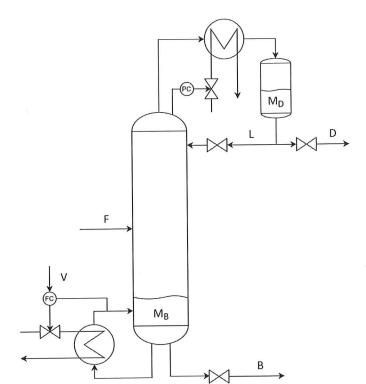
The feed and its composition are given by the upstream processes and outside of our analysis. The pressure in the column is controlled by the coolant flowrate and is deemed constant.
