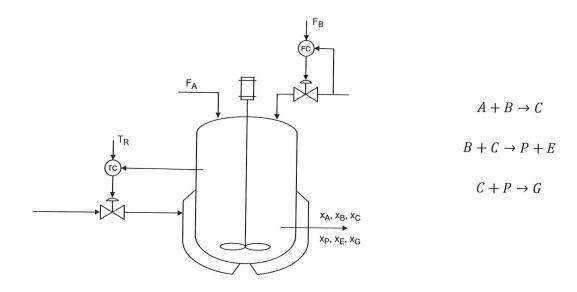
The feed stream  $F_A$ , with pure A component, is a given disturbance to the process. The process has two degrees of freedom, namely  $F_B$  and the reactor temperature  $T_R$ , shown in red in the figure above. The objective is to maximize the production of the valuable products P and E, subject to purity constraints on G and A.
