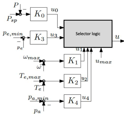
There is a PI controller to control each of the outputs using the single MV, as shown in the figure below, and one needs to select a value from the different controllers using maximum, minimum or mid selector blocks. However, the engineer is not sure how to design the selector block to automatically switch between the different controllers.
