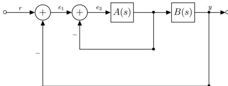
1. Derive the transfer function  $T(s)$  from  $r \rightarrow y$ .
