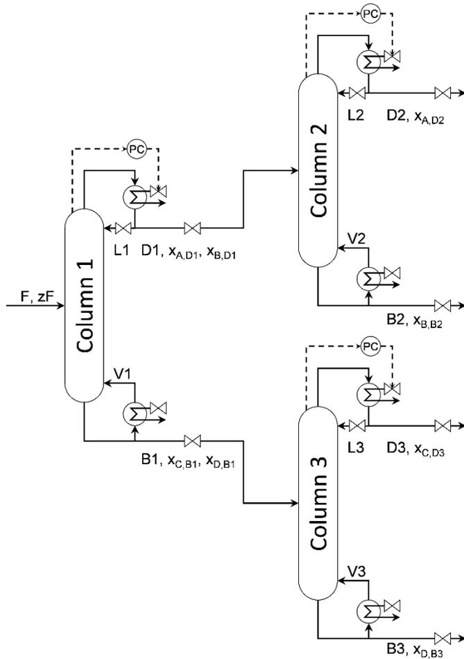
The feed and its composition are given by the upstream processes and our outside of the analysis. The pressure in each column is controlled by the coolant flowrate (see figure).
