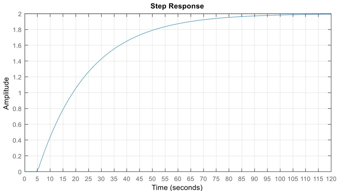
Assuming perfect measurements (i.e. no additional measurement delay), design a PI controller when  $\tau_c = \theta$ .
