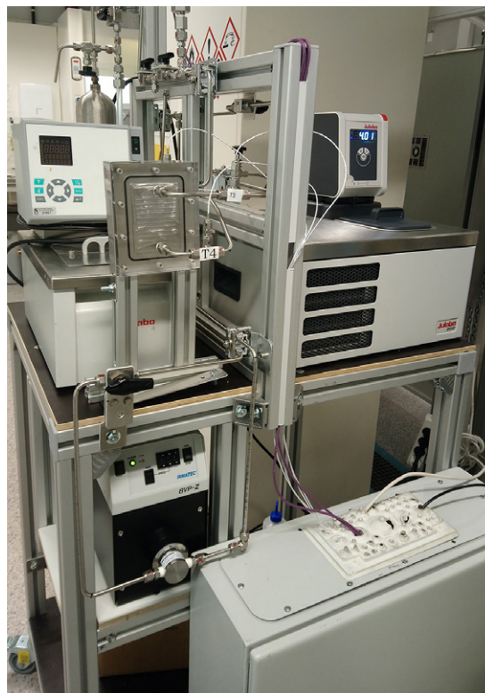
Figure 1. Thermopervaporation test rig for glycol regeneration.
