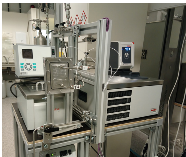
Thermopervaporation test rig for glycol regeneration.
