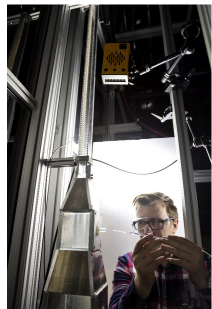
Test rig for study of particle breakup with droplet generation section (lower chamber) and droplet breakage section (upper column).
