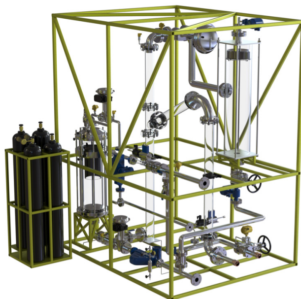
Subsea control system test rig with Gas liquid cylindrical cyclones, Compact flotation separator and associated pump system.
