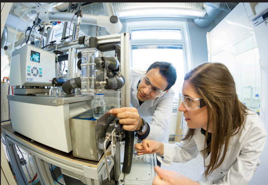
PhD students Mahdi Ahmadi and Eirini Skylogianni working with the membrane thermopervaporation setup for gas dehydration testing.
