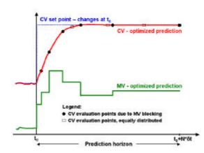
Fig. 1. MV blocking and CV evaluation
