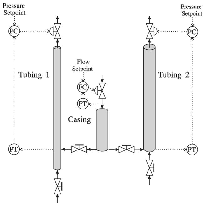
**Fig. 7—Controller structure for stabilization of the gas-distribution instability.**
