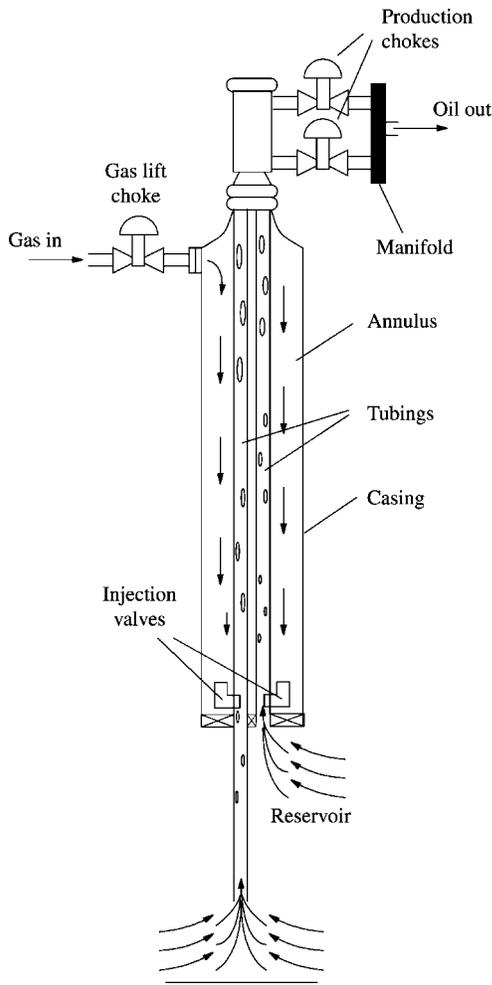
Fig. 1—A single-point dual gas lift oil well.
