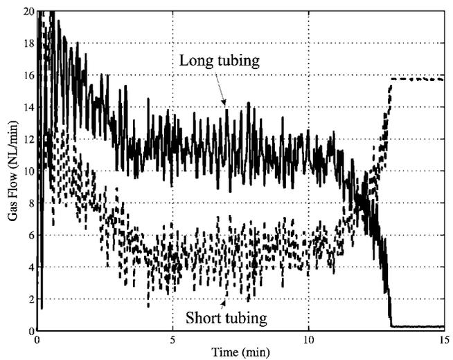
Fig. 16—Gas distribution as a function of time. Control is turned off at  $t=10$  minutes.
