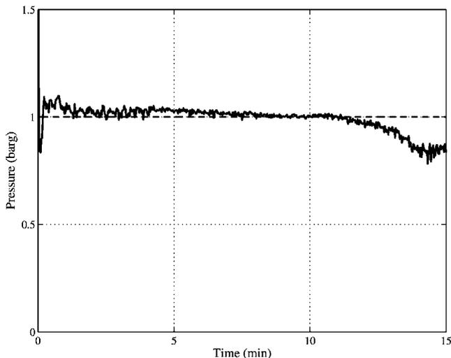
Fig. 13—Pressure at the location of gas injection in the short tubing. Control is turned off at  $t=10$  minutes. The dashed line specifies the setpoint  $p_{wi,2}^*$ .
