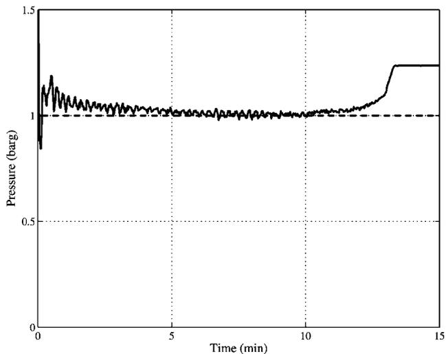
Fig. 12—Pressure at the location of gas injection in the long tubing. Control is turned off at  $t=10$  minutes. The dashed line specifies the setpoint  $p_{wi,1}^*$ .
