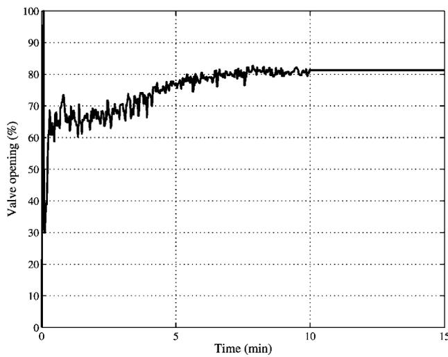
Fig. 15—Production-valve opening for the short tubing. Control is turned off at  $t=10$  minutes, keeping the valve opening at the last controlled value.
