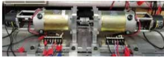
Figure 4. Photograph of the experimental two-mass resonance model.
