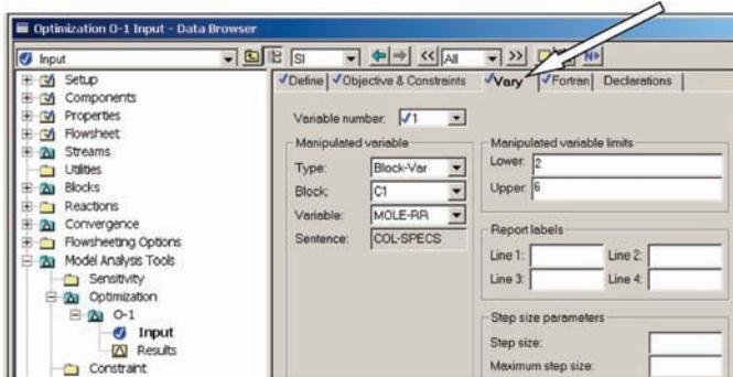
Figure 4.8 Specifying reflux ratio to vary.
