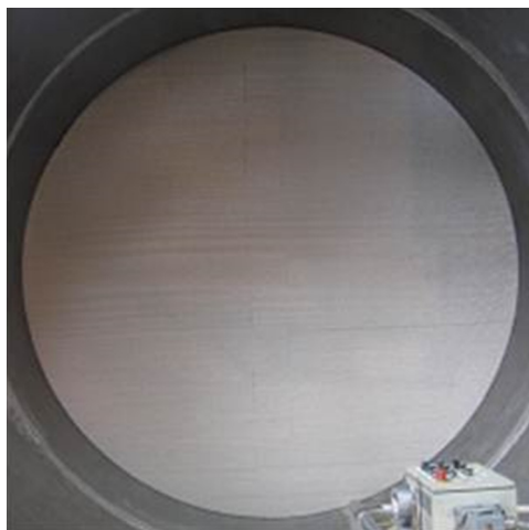
FIGURE 6.35 Photograph (c. 2002) of a Shop-Mounted Packed-Column Section with Segmented Packing Stripes and Reduced Gaps at the Junction of the Divided Elements.
