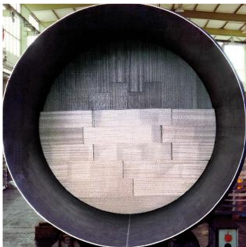
FIGURE 6.34 Photograph (c. mid-1990s) of a Shop-Mounted Packed-Column Section with Filled Gaps at the Junction of the Segmented Packing Stripes.
