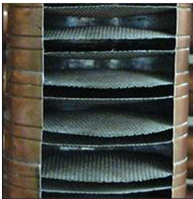
FIGURE 6.10 Lens-like dual-flow tray in one of the first air distillation columns.
