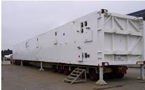
FIGURE 6.6 Photograph of a Transportable Packaged Unit Containing the Pressure Column, Main Condenser, and the Low-Pressure Column.
