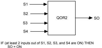
IF (at least 2 inputs out of S1, S2, S3, and S4 are ON) THEN SO = ON ELSE SO = OFF
