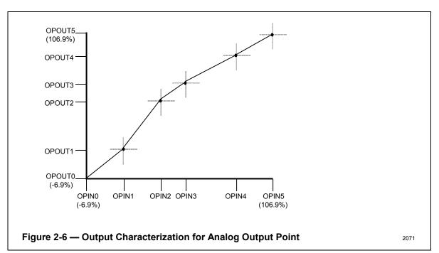
Depending on the output value, the analog output point interpolates linearly between the two nearest values. The interpolated value becomes the output value OPFINAL.
