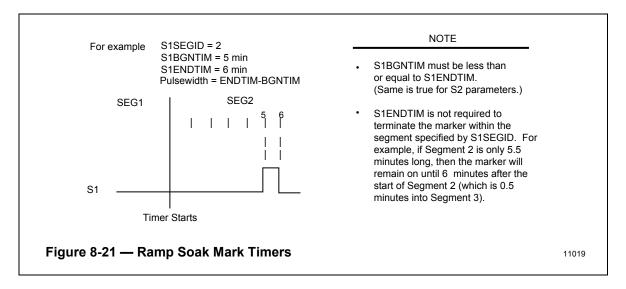
The S1 or S2 flag is turned on at the number of minutes after the specified segment begins, as is specified in SnBGNTIM. The corresponding flag is turned Off at the number of minutes after the specified segment begins, as specified in SnENDTIM.
