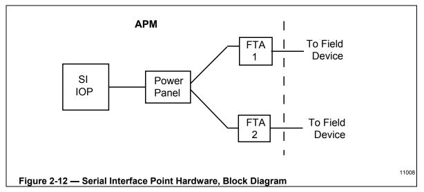
Communications to the field device is by EIA RS-232D or EIA RS-485 standards\*. RS-232D communication has a limit of 15 meters (50 feet) and RS-422/485 protocol is supported to 1.2 km (4000 feet). You can extend EIA RS-232D Communications between an FTA and a field device with appropriate MODEMs.
