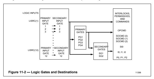
You can designate up to 12 Logical inputs (NOLINPTS) and enter an 8-character ASCII descriptor for each input (LIDESC(n) where n is 1–12). The ASCII descriptor can be changed by a CL program or a person with Engineer access level.
