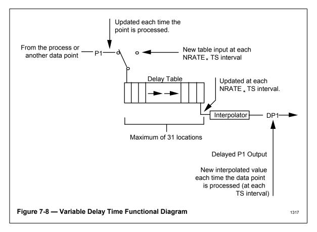
For an example of the delay-table operation, suppose that the P1-input value has been constant at 5.0 units for an hour. Assume that the specified delay time, TD, is 15 minutes and that the data point is processed every second; Time Sample (TS = 1/60) min. as determined by the SCANRATE parameter. At this time, the output of the interpolator is 5.0 units, all of the locations in the table contain a value of 5.0 units, and P1 contains a value of 5.0 units.
