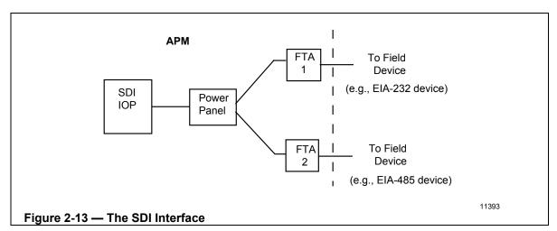
Figure 2-13 illustrates the Serial Device Interface.
