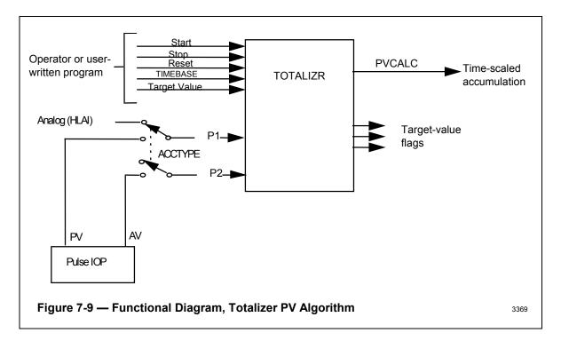
The accumulation can be started, stopped, and reset by commands from a Universal Station operator or from a user-written program. An operator or user-written program can establish a target value for the accumulation. Status indicators are available to indicate that the accumulation is near the target value, nearer to the target value, and is complete (has reached or exceeded the target value).
