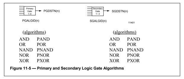
**Primary Gate Destinations**—Parameter PGDSTN(n) directs outputs from Primary Gate n to any <u>one</u> of the destinations shown in Figure 11-6.
