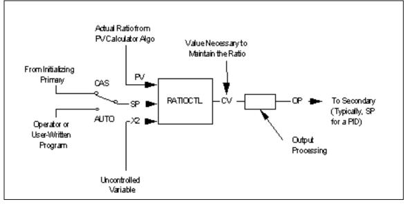
Figure 8-15 — Functional Diagram, Ratio Control Algorithm
