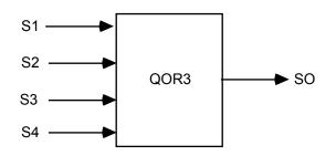
IF (at least 3 inputs out of S1, S2, S3, and S4 are ON) THEN SO = ON ELSE SO = OFF
