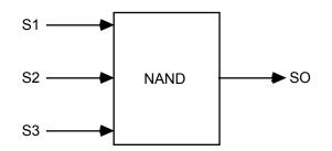
SO = NOT ( (((S1REV = OFF) AND (S1 = ON)) OR ((S1REV = ON) AND (S1 = OFF))) AND (((S2REV = OFF) AND (S2 = ON)) OR ((S2REV = ON) AND (S2 = OFF))) AND (((S3REV = OFF) AND (S3 = ON)) OR ((S3REV = ON) AND (S3 = OFF))))
