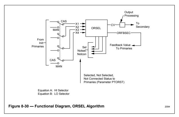
In a strategy like that of Figure 8-31, Equation A, the override option is configured. PID data points connected to non-selected inputs are prevented from "winding up" by forcing their outputs to track the override feedback signal (ORFBSEC). For more detail on such strategies, refer to 8.13.
