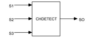
SO = (S1 < > S1\_last\_time) OR (S2 < > S2\_last\_time) OR (S3 < > S3\_last\_time)
