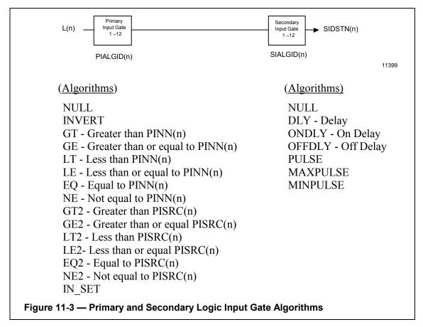
**Secondary Input Gate Algorithms**—These include various types of delays. Your entry (0 - 8000 seconds) in parameter SIDLYTIM(n) determines the delay (per gate). These functions are briefly described here and fully in the Logic Point description (Section 5).
