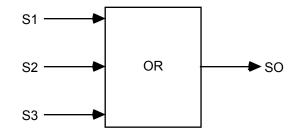
SO = (((S1REV = OFF) AND (S1 = ON)) OR ((S1REV = ON) AND (S1 = OFF))) OR (((S2REV = OFF) AND (S2 = ON)) OR ((S2REV = ON) AND (S2 = OFF))) OR (((S3REV = OFF) AND (S3 = ON)) OR ((S3REV = ON) AND (S3 = OFF)))
