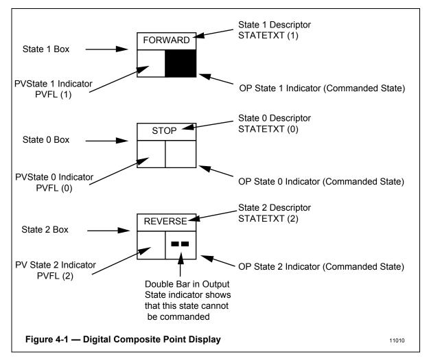
As an example, assume that the digital composite point shown in Figure 4-1 is connected through digital output points and digital input points to a motor control circuit and that the current state of the digital composite point is state 0 (STOP).
