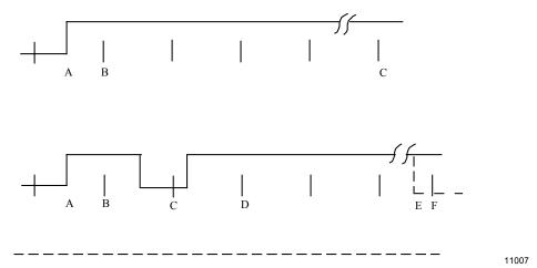
This waveform represents the field input. Tick marks across the waveform indicate the 200 microsecond scan intervals of the DISOE IOP hardware. Assume that the input state changes at point A.
