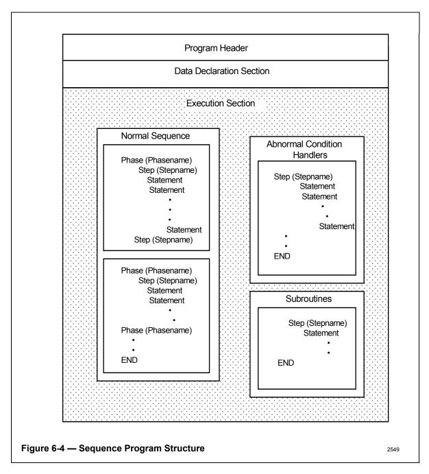
• *Subroutines*—Subroutines simplify the program structure and are used for executing repetitive functions, thereby reducing the programming effort and memory requirements. Subroutines can be called by the normal sequence, other subroutines, or abnormal condition handlers. Two levels of nesting are supported for both normal and abnormal sequences. A runtime error is generated if the nesting level is violated.
