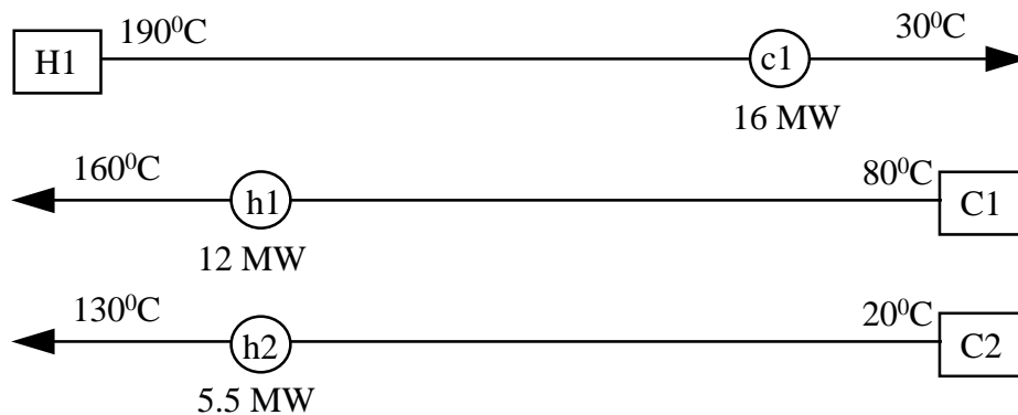
Figure 2.3 Trivial solution using external utilities only.
