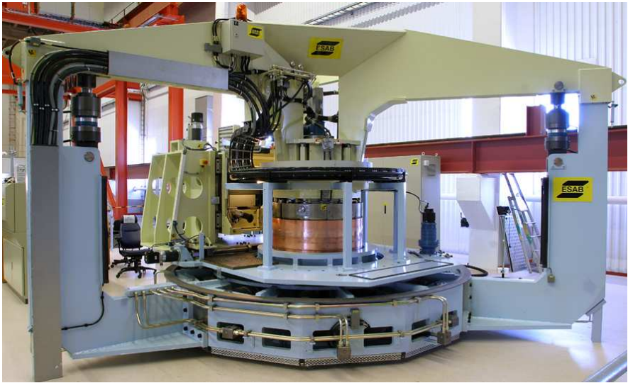
Figure 3. Purpose-built FSW machine for copper canister welding.
