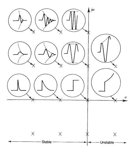
Figure 2.1: Relationship between pole position and transient response (Golten and Verwer, 1991)
