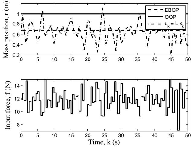
Figure 6.4: Time series plot of a mass spring damper system showing the performance of multivariable controller,  $u_k = L_d x_k$
