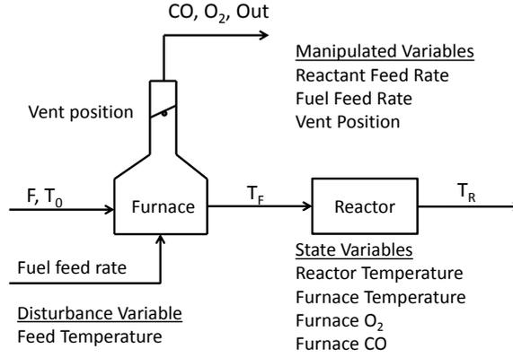
Figure 5.6: Preheating furnace reactor system
