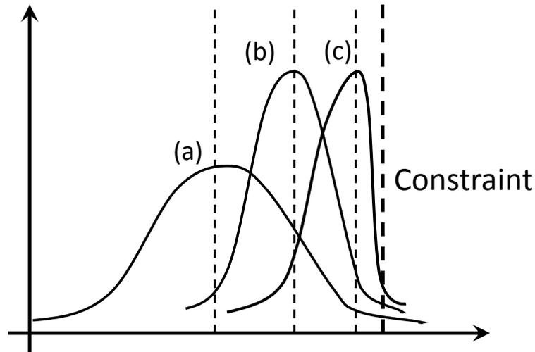
Figure 1.2: Set point selection showing performance of - (a) a badly tuned linear controller, (b) a well tuned linear controller, and (c) a well tuned non-linear controller
