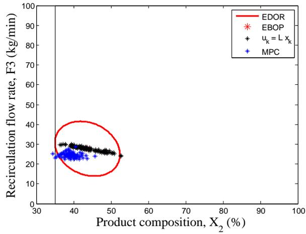
Figure 6.7: Scatter plot showing the EDOR between product composition vs recirculation flow rate
