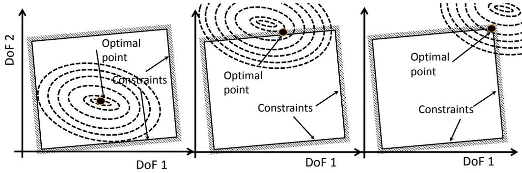
Figure 1.3: Nature of optimal solutions - unconstrained; partially constrained; fully constrained optimum
