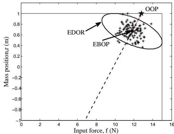
Figure 6.3: Scatter plot of a mass spring damper system showing the performance of MPC controller
