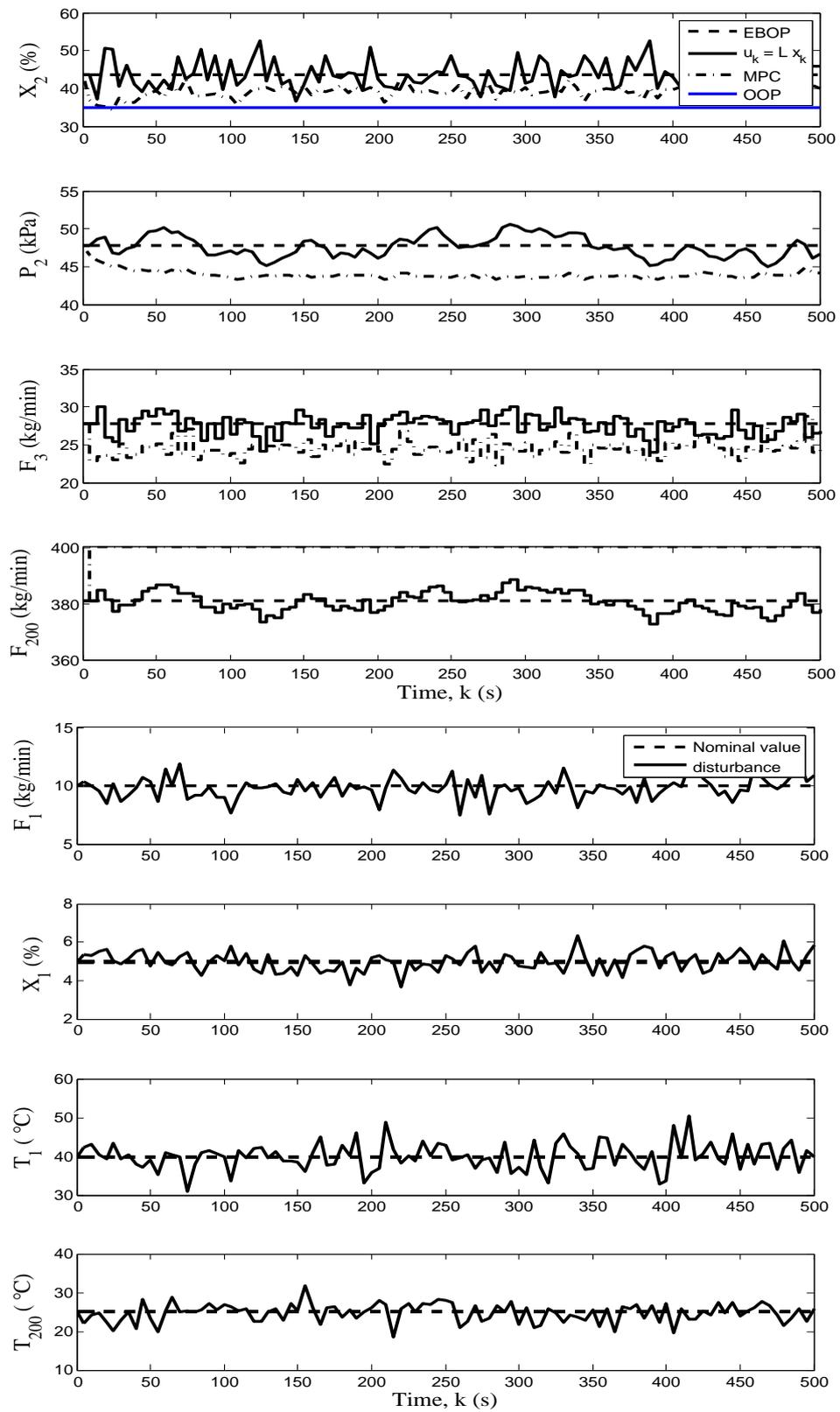
Figure 6.10: Time-series plot of the evaporation process showing the controller performances at the economic back-off point
