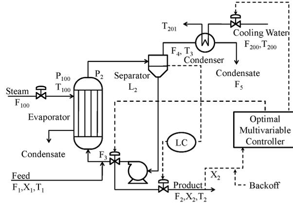
Figure 5.13: Evaporator system
