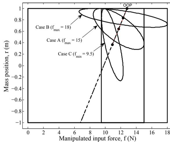
Figure 5.5: Impact of change in constraint for mass spring damper system
