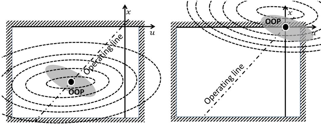
Figure 1.4: Process operation under uncertain conditions in input-output space at unconstrained and constrained optimum
