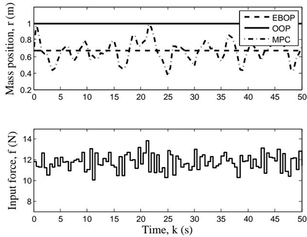
Figure 6.5: Time series plot a mass spring damper system showing the performance of MPC controller
