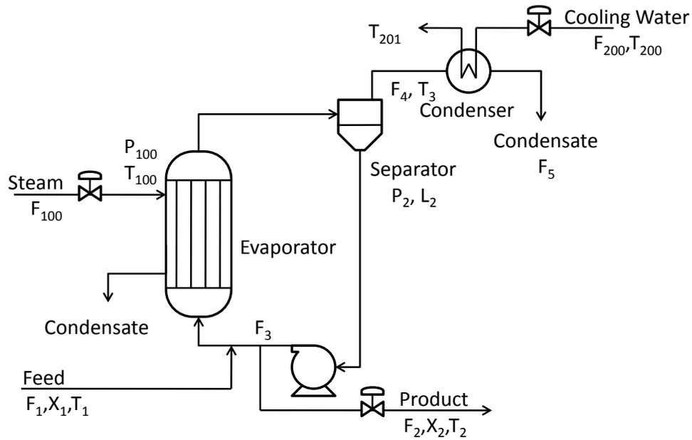
Figure 3.1: Evaporator system
