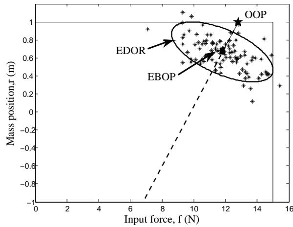
Figure 6.2: Scatter plot of a mass spring damper system showing the performance of multivariable controller,  $u_k = L_d x_k$
