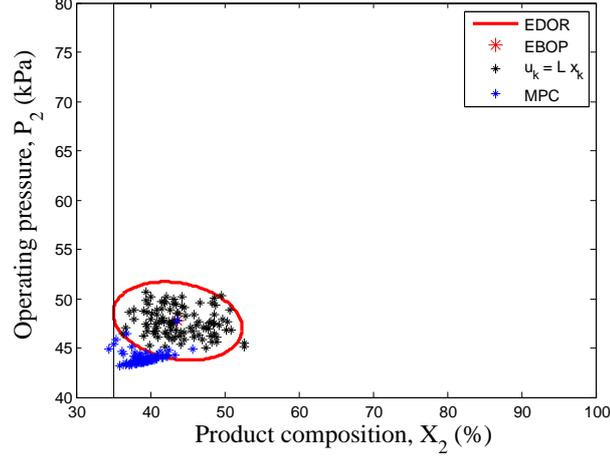
Figure 6.6: Scatter plot showing the EDOR between product composition vs operating pressure
