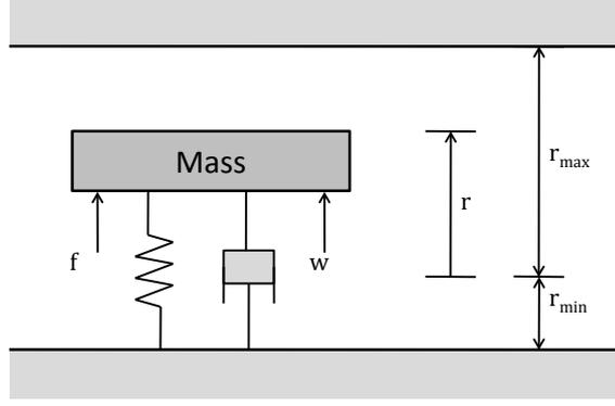
Figure 5.4: Mass spring damper system
