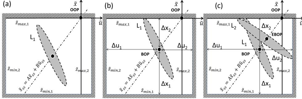
Figure 6.1: Two stage iterative solution approach for economic back-off selection: (a) stage 1 solution; (b) stage 2 solution; (c) converged stage 2 solution
