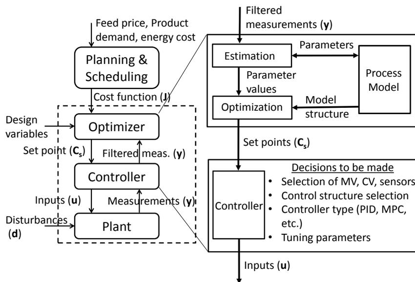
Figure 1.1: Hierarchical structure of plant operations based on time scale separation showing the set of decisions involved in optimization and control layer
