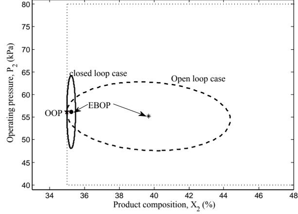
Figure 5.14: Product composition vs operating pressure. a) Open loop case:  $F_3$  and  $F_{200}$  are constant. b) Closed loop case:  $F_3$  and  $F_{200}$  are used for control of  $X_2$
