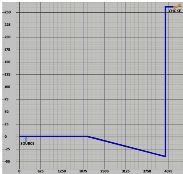
Figure 2.2: Geometry of OLGA pipeline-riser test case
