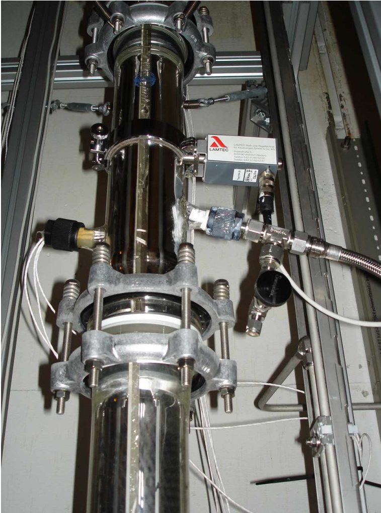
Figure 9.2: Sidestream product draw. Swinging funnel inside column section directs the liquid to the product line or as reflux.
