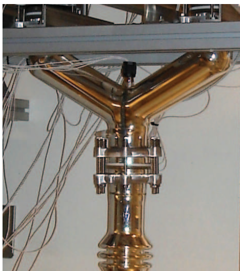
Figure 8.2: The top of the bottom section where the column splits into the prefractionator (left) and main column. Flooding was a problem in this section of the column.
