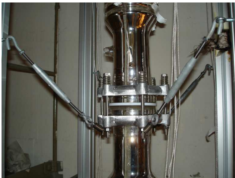
Figure 7.3: Springs and turnbuckles help centering the column and compensates for the weight of each column section.
