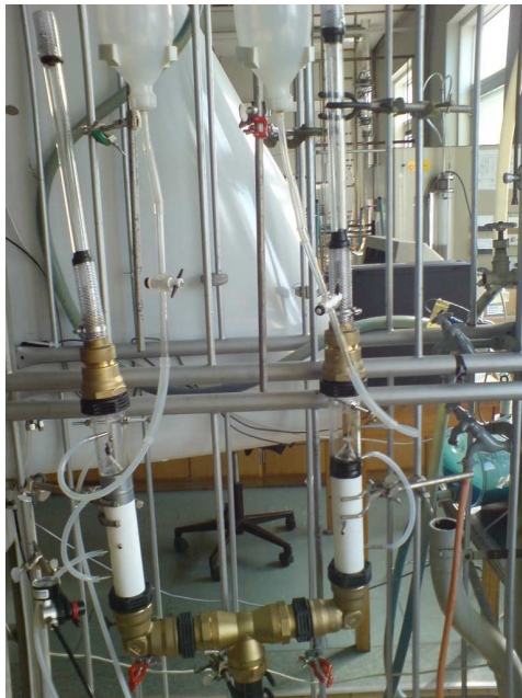
Figure 7.7: Rig for testing new valve solutions using air and water
