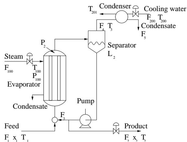
Figure 4.1: Evaporation process
