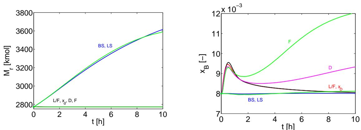
Figure 3.16: Reactor holdup ( $M_r$ ) (left) and product composition ( $x_B$ ) (right) when  $\Delta F_0 = +20\%$  with nominal setpoints.
