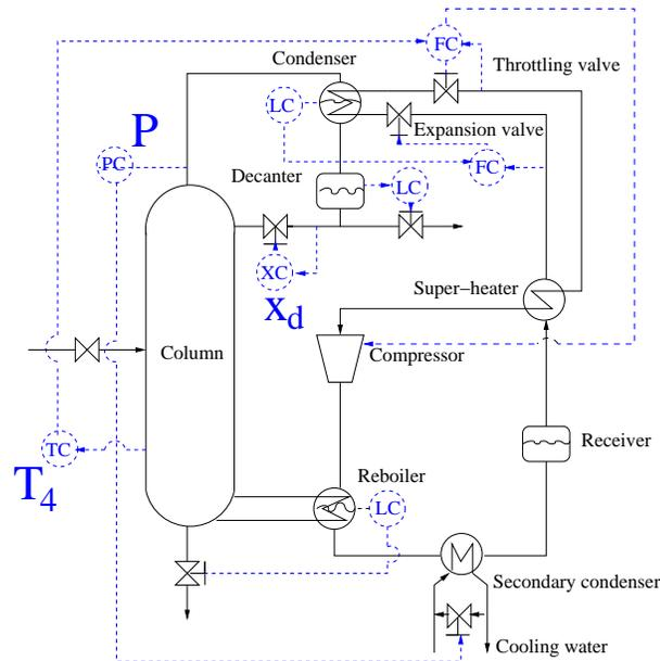
Figure 6.2: Distillation column with heat pump with proposed control structure
