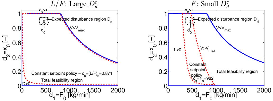
Figure 3.18: The constant setpoint policy feasibility region (dashed) when controlling  $L/F$  with nominal setpoints ( $D_d^{nom,L/F} = \{\tilde{D}_{dc}^{nom,L/F} | d_c = d_{c,max}^*\}$ ) (left) and when controlling  $F$  with nominal setpoints ( $D_d^{nom,F} = \{\tilde{D}_{dc}^{nom,F} | d_c = d_{c,max}^*\}$ ) (right).
