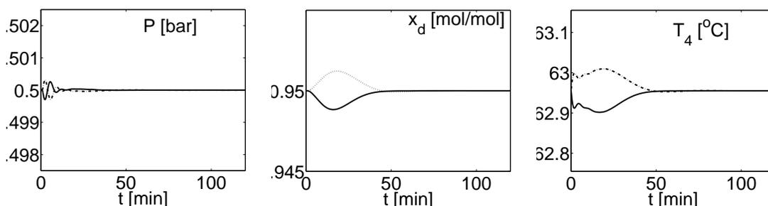
Figure 6.3: Column pressure ( $p$ ), top composition ( $x_D$ ) and temperature at stage 4 ( $T_4$ ) for steps in the feedrate ( $F$ ). (Solid shows a 20% increase in  $F$  and dashed shows a 20% decrease in  $F$ .)
