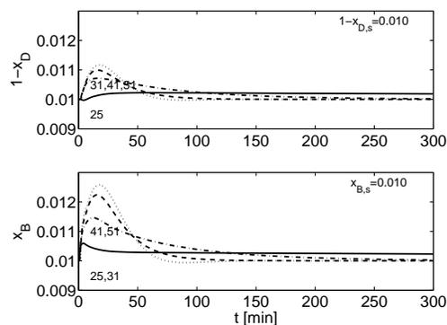
Figure 7.16: Output responses to 10% increase in  $z_F$  with SIMC-tuned PI-controllers.
