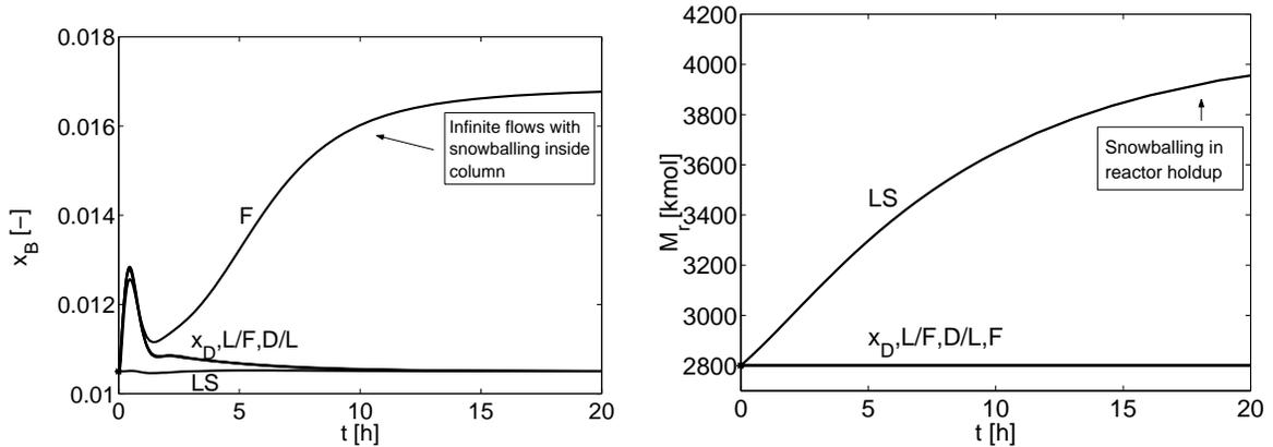
Figure 2.8: Dynamic responses in  $x_B$  (left) and  $M_r$  (right) to a 20% step increase in  $F_0$  (Case I) for alternative control structures
