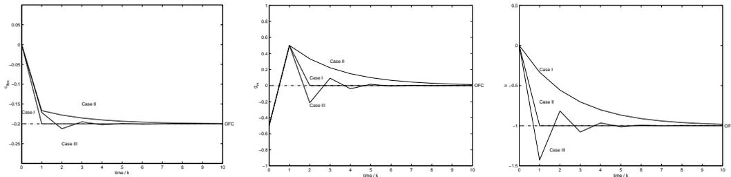
Figure B.1: The flexible setpoints ( $c_{flex}$ ), measured constraints ( $g_m$ ) and input  $u$  as function of time for case I, II and III.
