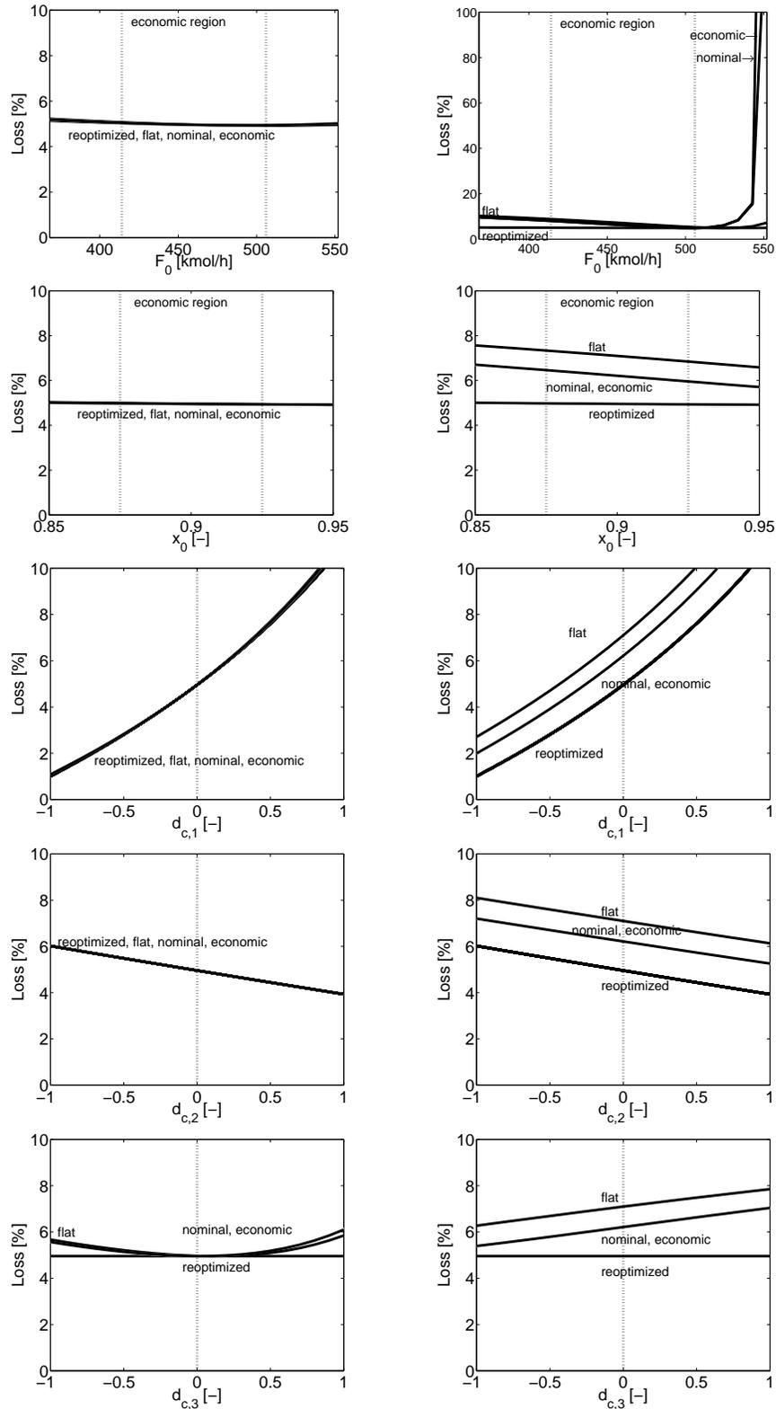
Figure A.4: Loss as function of disturbances ( $F_0$ ,  $x_0$ ) and implementation errors ( $d_{c,1}, d_{c,2}, d_{c,3}$ ) for constant robust setpoints based on the flat cost, nominal cost and economic approach when controlling  $L/F$  (left column) and  $F$  (right column).
