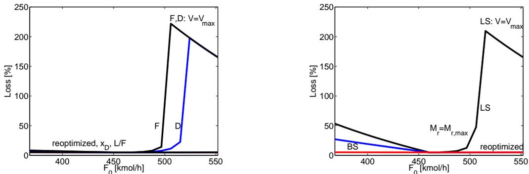
Figure 3.15: Loss with flexible setpoints as a function of disturbance  $F_0$  for "good" controlled variables (left) and "poor" controlled variables (right).
