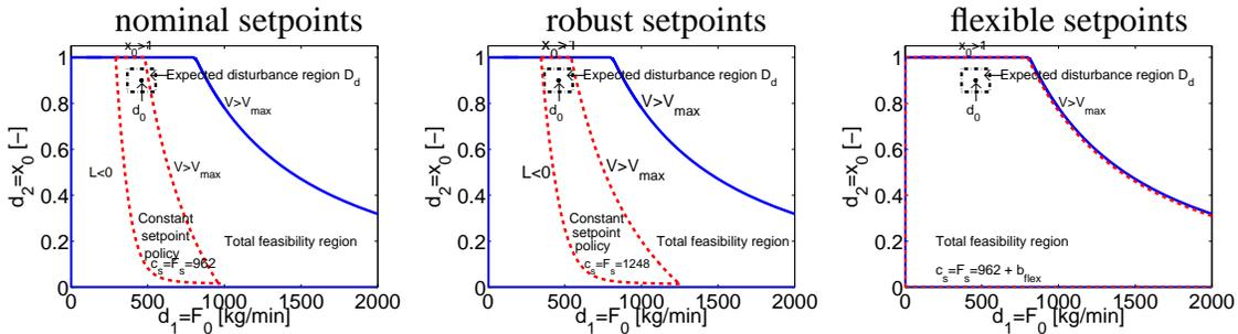
Figure 3.19: The feasibility region (dashed) with constant nominal setpoints (left), constant robust setpoints (middle) and flexible setpoints (right) when controlling  $F$  and with implementation errors  $d_c = d_{c,max}^*$ .
