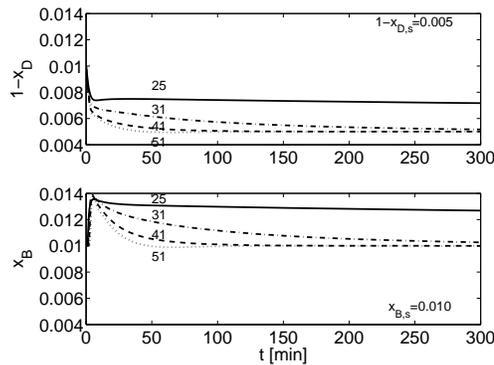
Figure 7.17: Output responses with a setpoint change in  $x_{D,s}$  from 0.990 to 0.995 with SIMC-tuned PI-controllers.
