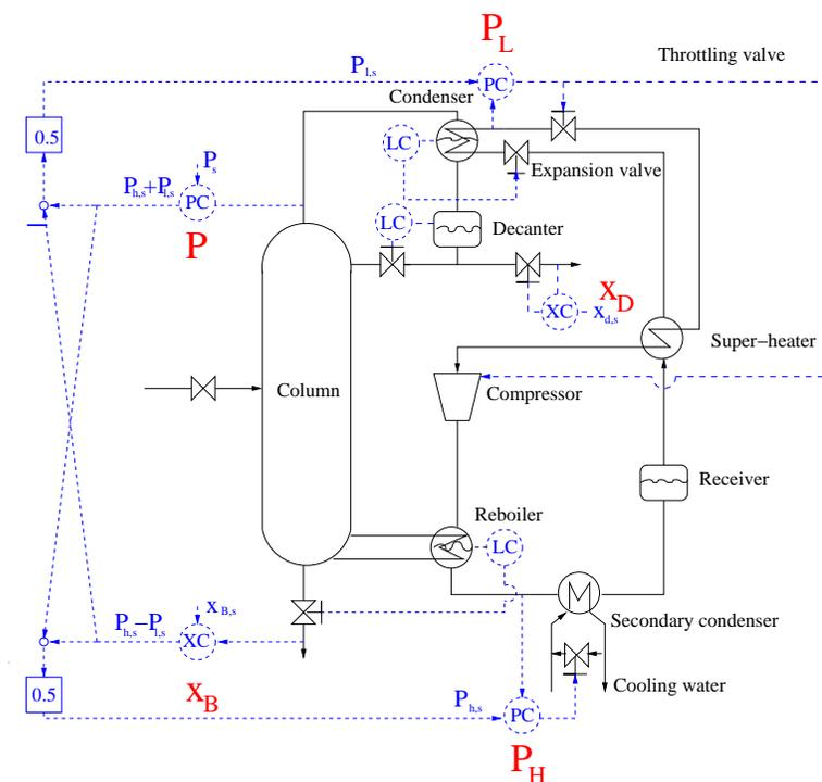
Figure 6.1: Distillation column with heat pump with proposed control structure in literature
