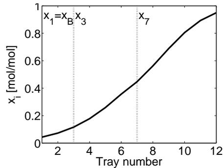
Figure 6.5: Composition profile in the distillation column
