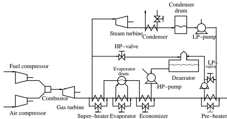
Figure 5.2: A simple combined cycle power plant process
