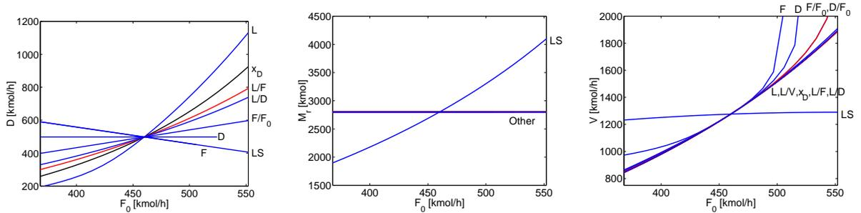
Figure 2.2: Snowballing: Steady-state values of the recycle flow ( $D$ ), reactor holdup ( $M_r$ ) and column boilup ( $V$ ) as a function of feedrate  $F_0$  for alternative control structures.
