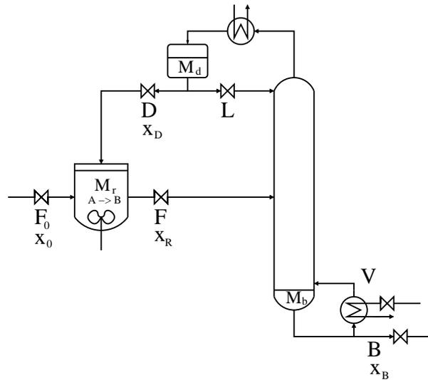
Figure 3.10: Reactor/separator process with liquid recycle
