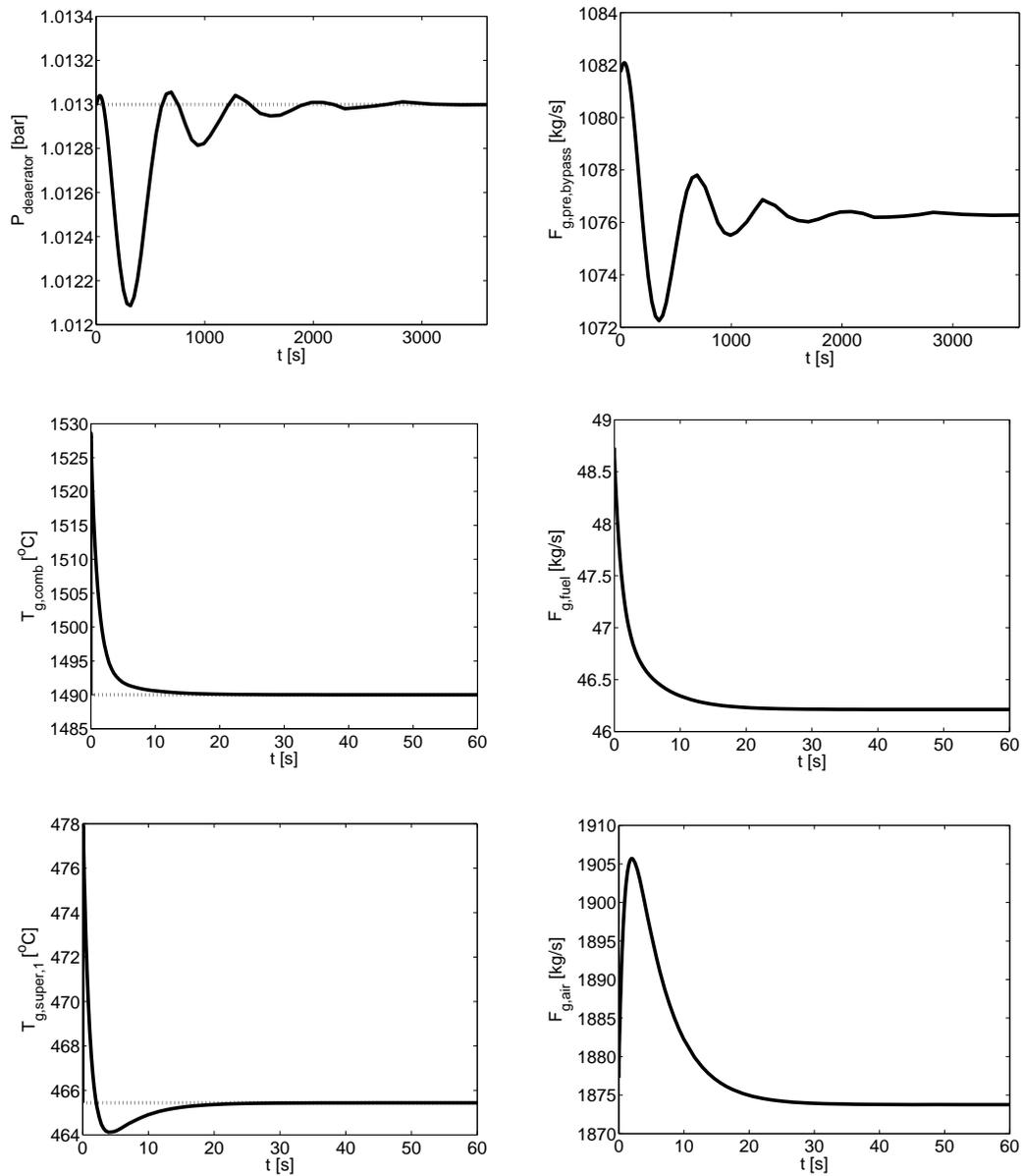
Figure 5.9: The deaerator pressure, pre-heater bypass flowrate, combustor temperature, fuel feedrate, super-heater gas inlet temperature and air feedrate response when increasing the feed air temperature with  $10^{\circ}\text{C}$
