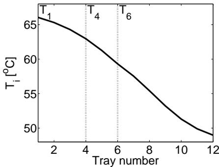
Figure 6.4: Temperature profile in the distillation column
