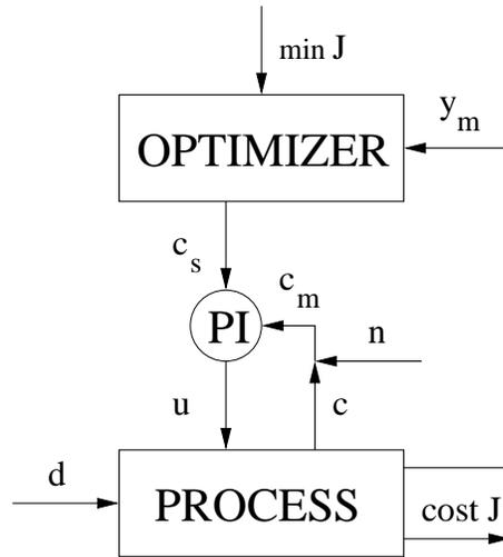
Figure 3.1: A typical optimization system incorporating local feedback: The process is disturbed ( $d$ ) and the control system tries to keep the controlled variables ( $c$ ) at their setpoints ( $c_s$ ). Steady-state optimization based on process measurements ( $y_m$ ) is performed at regular intervals to track the optimum by updating the setpoints.
