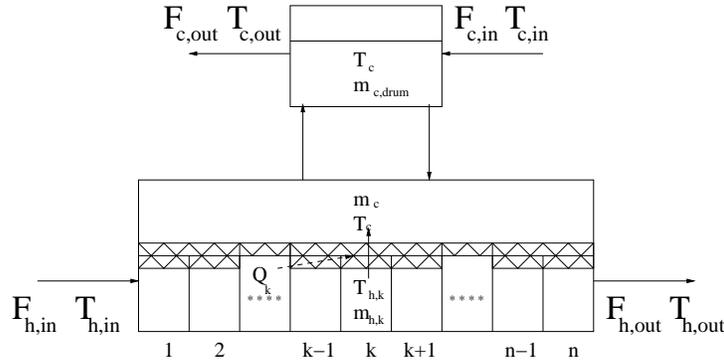
Figure C.4: Heat exchanger model II (heat-exchanger with drum)
