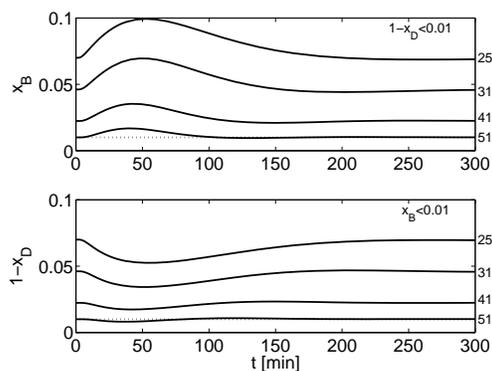
Figure 7.22: Responses with over-purification for a 10% increase in  $z_F$ . Nominal boilup  $V=2.73$  kmol/min in all cases.
