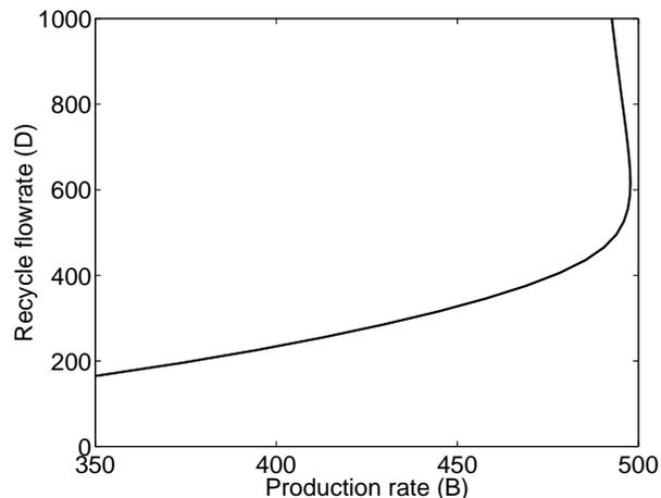
Figure 2.5: Snowballing with  $V$  constant: Recycle flow  $D$  as a function of production rate  $B = F_0$  (Case II,  $M_r = 2800$ ,  $x_B = 0.0105$ ,  $V = 1400$ ).
