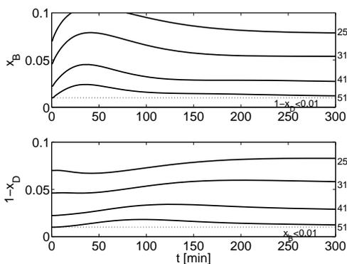
Figure 7.21: Responses with over-purification for a 10% increase in  $F$ . Nominal boilup  $V=2.73$  kmol/min in all cases.
