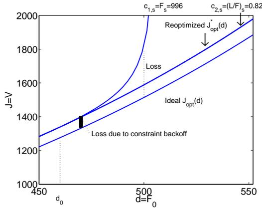
Figure 3.6: Cost as a function of disturbance  $d$  with (i) ideal optimization (lower curve), (ii) reoptimization with constraint backoff and (iii) two different constant setpoint policies ( $c_1$  and  $c_2$ ). The loss is negligible with  $c_2$  as a controlled variable. The loss due to constraint backoff is unavoidable if we want to guarantee feasibility.
