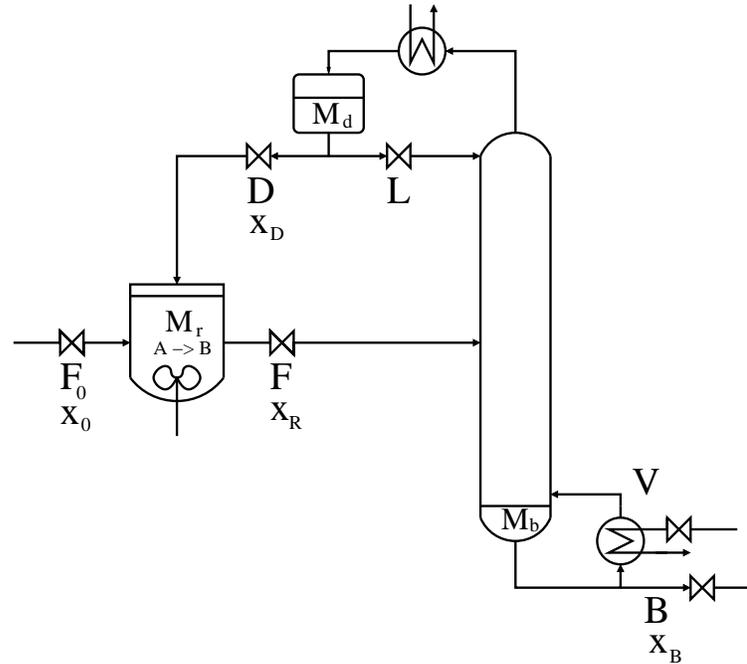
Figure 2.1: Reactor, separator (distillation) and recycle process.
