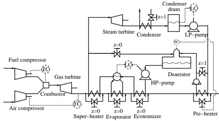
Figure 5.6: Combined cycle power plant process with proposed control structure for case III
