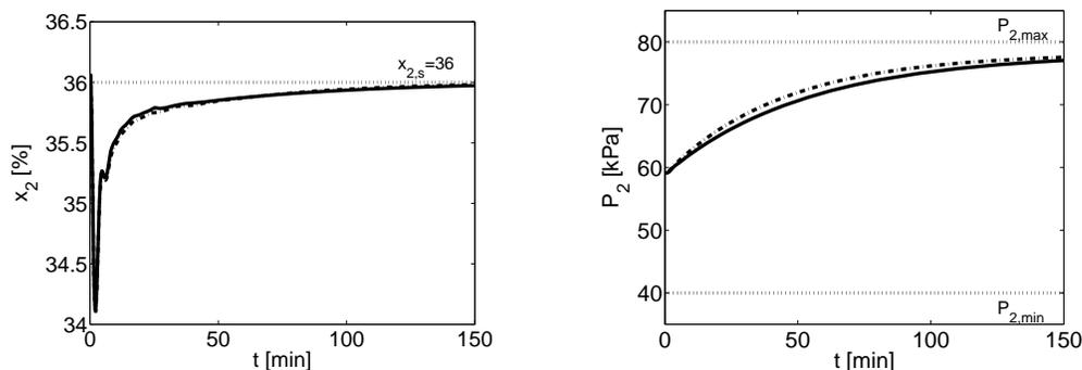
Figure 4.7:  $x_2$  and  $P_2$  when controlling either  $F_{200}/F_1$  (solid) or  $T_{201} - T_{200}$  (dashed) with constant robust setpoints and  $F_1$  increased with 20% (from 10 kg/s to 12 kg/s).
