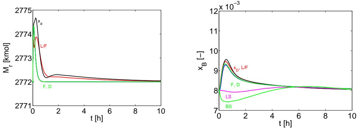
Figure 3.17: Reactor holdup ( $M_r$ ) (left) and product composition ( $x_B$ ) (right) when  $\Delta F_0 = +20\%$  with robust setpoints.
