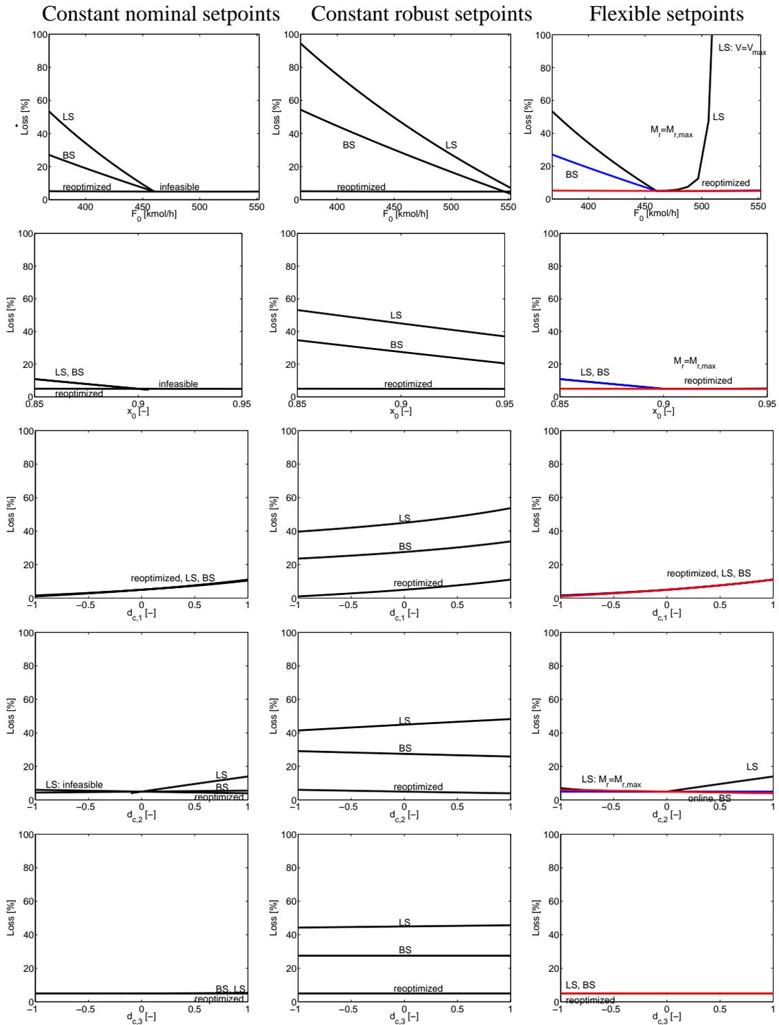
Figure 3.14: Loss as a function of disturbances ( $F_0, x_0$ ) and implementation errors ( $d_{c,1}, d_{c,2}, d_{c,3}$ ) for the "poor" controlled variables.
