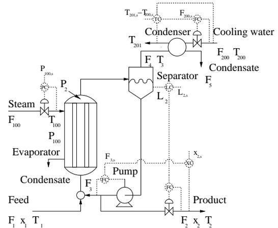
Figure 4.6: Evaporation process with control structure when controlling  $T_{201} - T_{200}$
