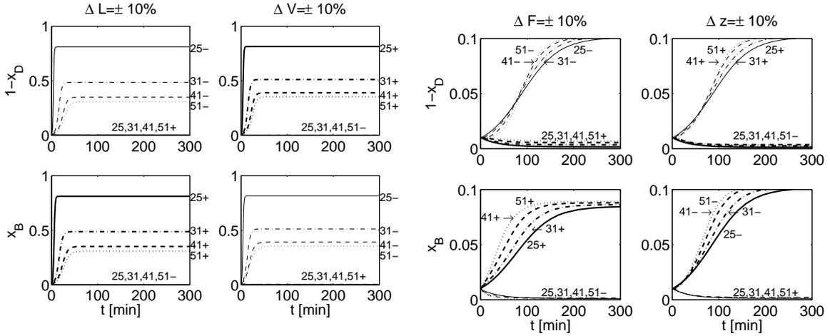
Figure 7.3: Open-loop output responses for steps in inputs (left side) and disturbances (right side)
