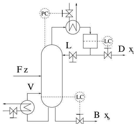
Figure 7.1: One-feed two-product distillation column
