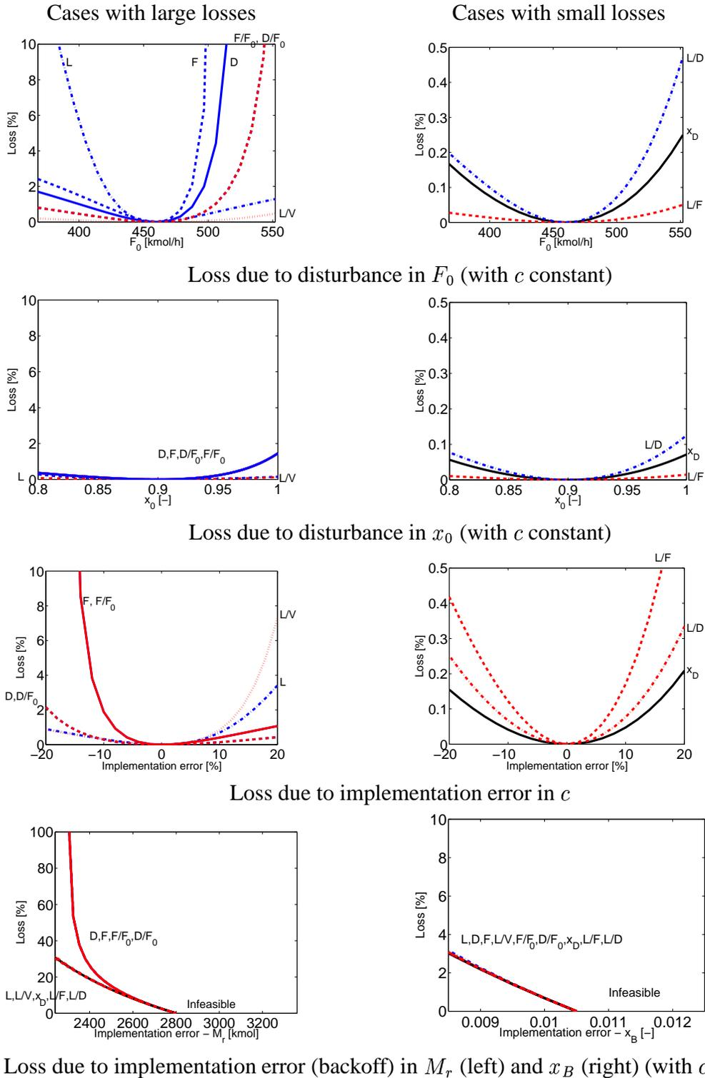
Figure 2.3: Case I: Losses in energy ( $V$ ) with alternative controlled variables ( $F_0 = 460$ ,  $M_r = 2800$ ,  $x_B = 0.0105$ ).
