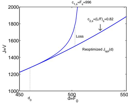
Figure 3.4: Cost as a function of the disturbance with (i) reoptimized setpoint (lower curve) and (ii) two alternative constant setpoint policies ( $c_1$  and  $c_2$ ). The loss is negligible with  $c_2$  as a controlled variable.
