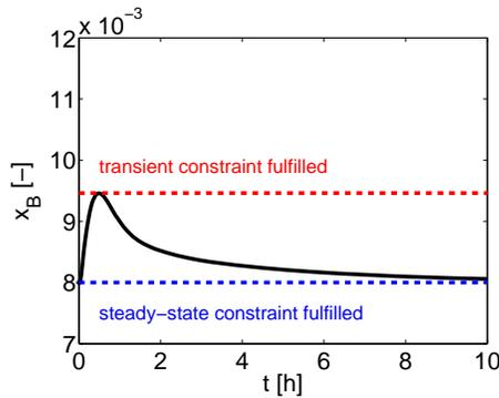
Figure 3.2: Fulfilled steady-state and transient constraint.
