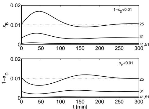
Figure 7.19: Responses with over-purification for a 10% increase in  $F$ . Nominal boilup  $V=22.0$  kmol/min in all cases.
