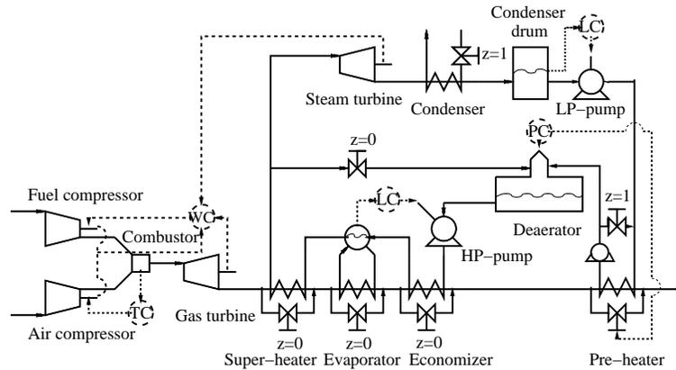
Figure 5.8: Combined cycle power plant process with proposed control structure for case II
