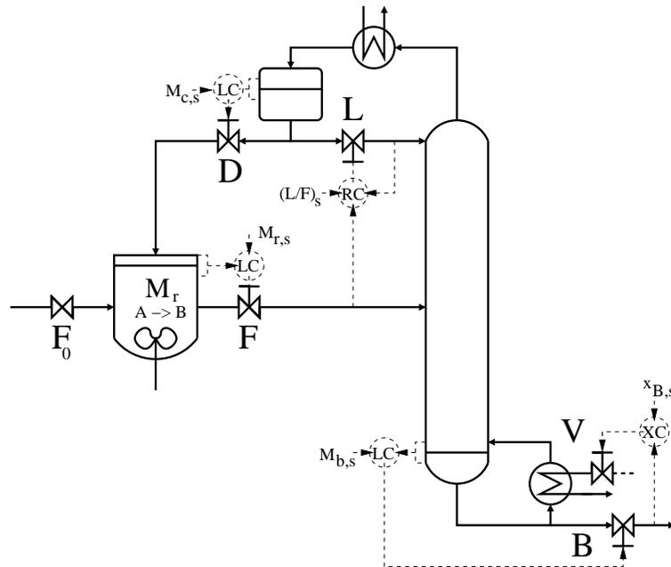
Figure 2.4: Reflux ratio control structure (Case I with given feedrate)
