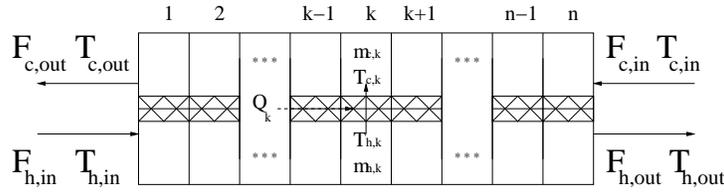
Figure C.3: Heat exchanger model I
