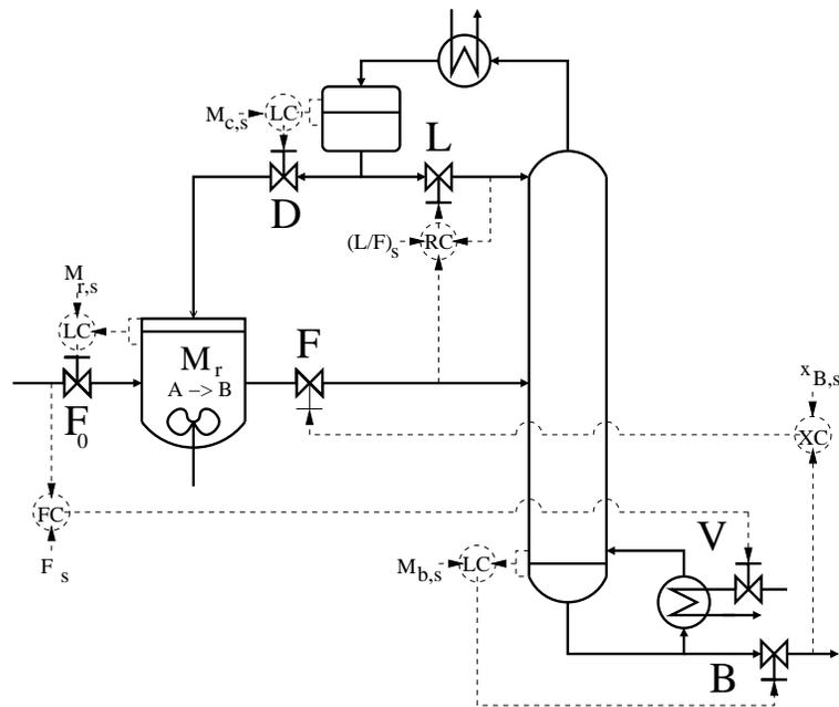
Figure 2.7: Reflux ratio control structure for case II (with flow control loop to handle also case I)
