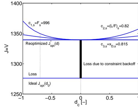
Figure 3.7: Cost as a function of implementation error. The loss is negligible with  $c_3$  as a controlled variable. The additional loss due to constraint backoff is unavoidable.
