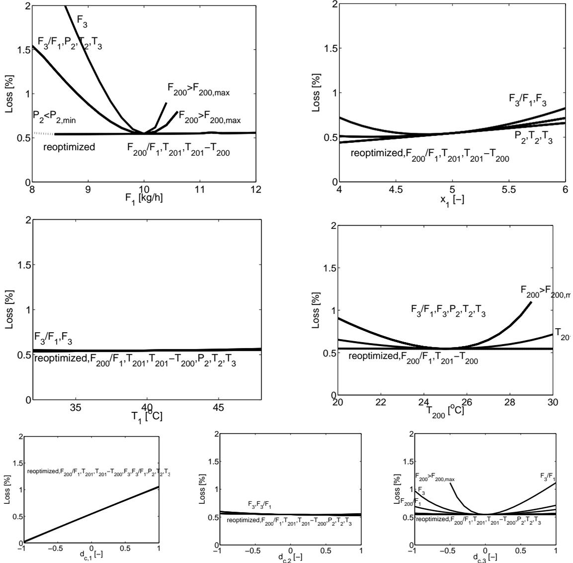
Figure 4.2: Loss as function of disturbances ( $F_1$ ,  $x_1$ ,  $T_1$ ,  $T_{200}$ ) and implementation errors ( $d_{c,1}, d_{c,2}, d_{c,3}$ ) with constant nominal setpoints ( $c_{s,0}$ ).
