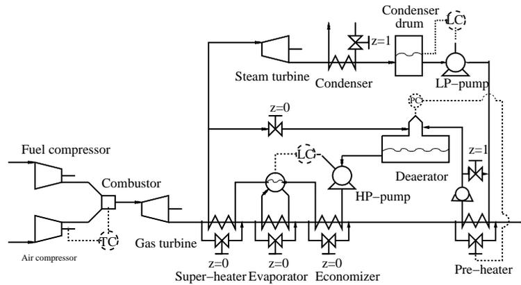
Figure 5.7: Combined cycle power plant process with proposed control structure for case I
