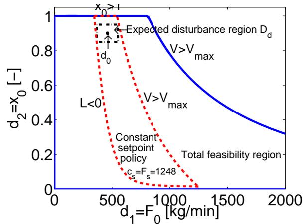
Figure 3.3: Total feasible region ( $D_d$ ) (solid), feasible region for a constant setpoint policy (controlling  $F$  with robust setpoints) ( $D_d^c = \{D_{dc}^{c,robust} | d_c = d_{c,max}^*\}$ ) (dashed) and expected disturbance region ( $D$ ) (dash-dot).
