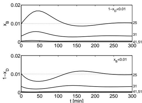
Figure 7.20: Responses with over-purification for a 10% increase in  $z_F$ . Nominal boilup  $V=22.0$  kmol/min in all cases.
