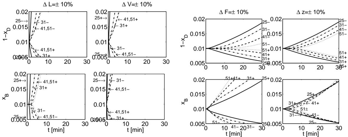
Figure 7.4: Initial open-loop output responses for steps in inputs (left side) and disturbances (right side)
