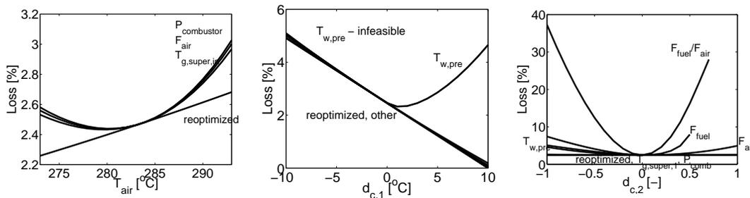
Figure 5.3: Loss as function of disturbances in the air feed temperature ( $T_{air}$ ), implementation error in controlling the combustor temperature  $T_{comb}$  ( $d_{c,1}$ ) and implementation error in the unconstrained controlled variable ( $d_{c,2}$ ).
