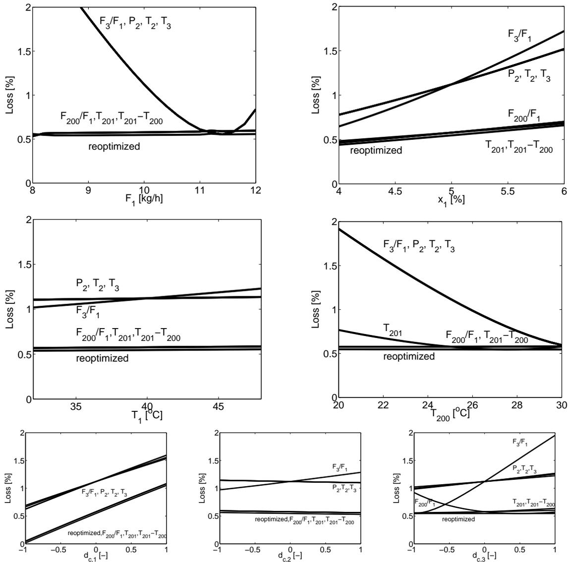
Figure 4.3: Loss as function of disturbances ( $F_1$ ,  $x_1$ ,  $T_1$ ,  $T_{200}$ ) and implementation errors ( $d_{c,1}, d_{c,2}, d_{c,3}$ ) with constant robust setpoints ( $c_{s,robust}$ ).
