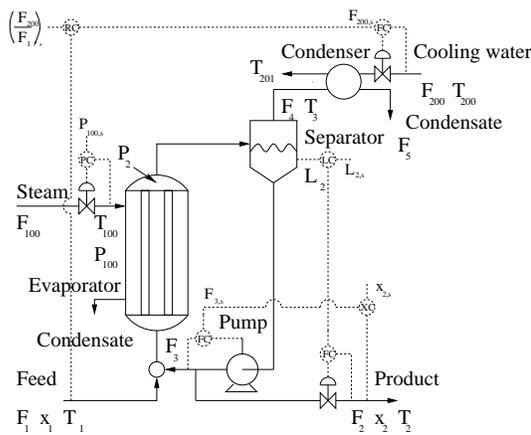
Figure 4.5: Evaporation process with control structure when controlling  $F_{200}/F_1$
