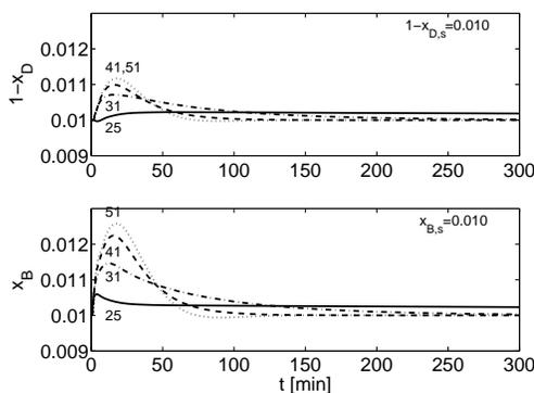
Figure 7.15: Output responses to 10% increase in  $F$  with SIMC-tuned PI-controllers.
