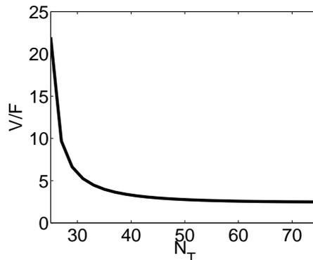
Figure 7.2: Nominal boilup as function of number of stages with fixed product purities ( $x_D = 0.99$ ,  $x_B = 0.01$ ).
