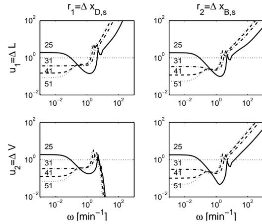
Figure 7.10: Input usage with perfect reference tracking ( $G^{-1}R(j\omega)$ )
