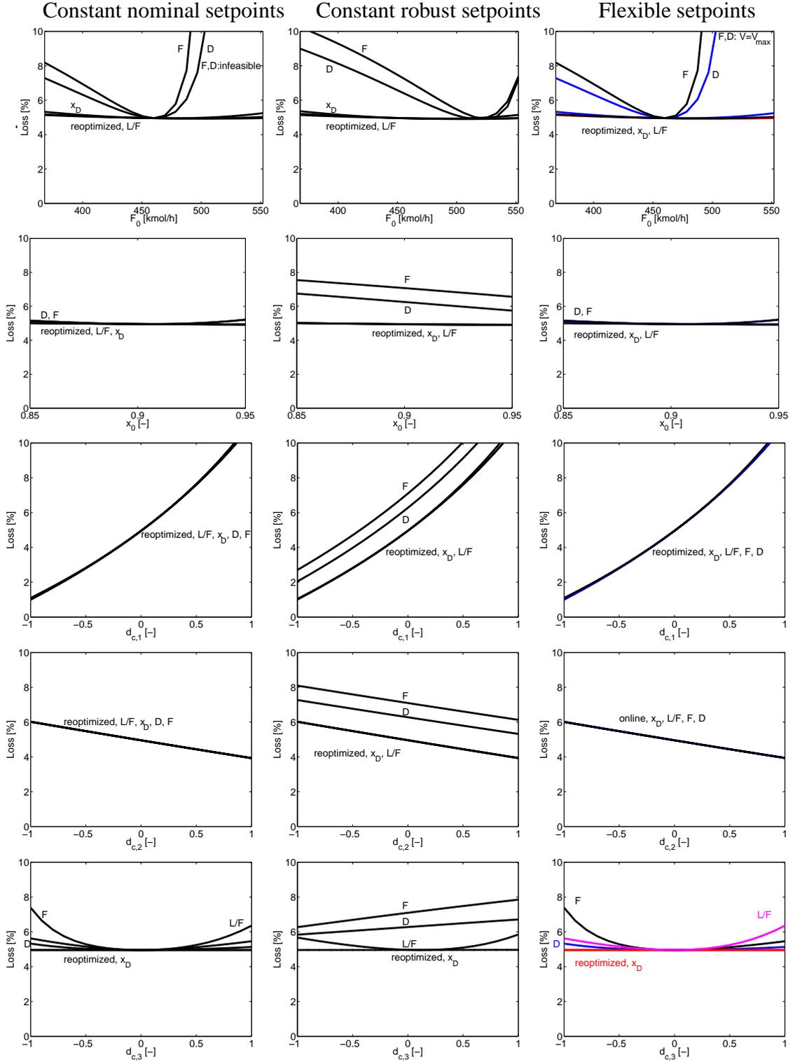
Figure 3.13: Loss as a function of disturbances ( $F_0$ ,  $x_0$ ) and implementation errors ( $d_{c,1}, d_{c,2}, d_{c,3}$ ) for the "good" controlled variables.
