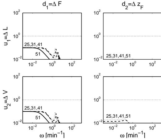
Figure 7.9: Input usage with perfect disturbance rejection ( $G^{-1}G_d(j\omega)$ )
