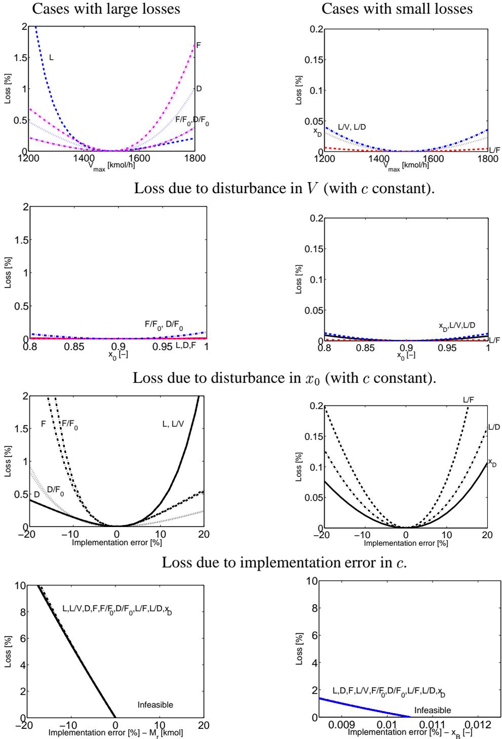
Loss due to implementation error (backoff) in  $M_r$  (left) and  $x_B$  (right) (with  $c$  constant).
