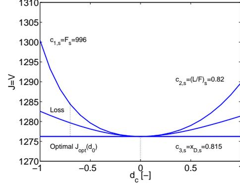
Figure 3.5: Cost as a function of the implementation error. The loss is negligible with  $c_3$  as a controlled variable.
