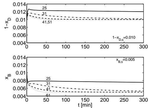
Figure 7.18: Output responses with a setpoint change in  $x_{B,s}$  from 0.010 to 0.005 with SIMC-tuned PI-controllers.
