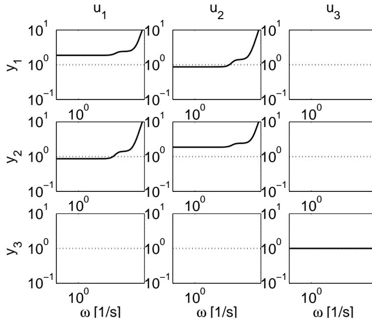
Figure 5.4: Frequency-dependent RGA ( $\Lambda(j\omega)$ )
