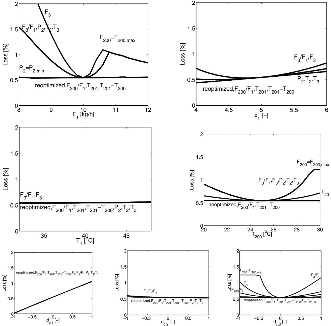
Figure 4.4: Loss as function of disturbances ( $F_1, x_1, T_1, T_{200}$ ) and implementation errors ( $d_{c,1}, d_{c,2}, d_{c,3}$ ) with flexible setpoints ( $c_{s,flex}$ ).
