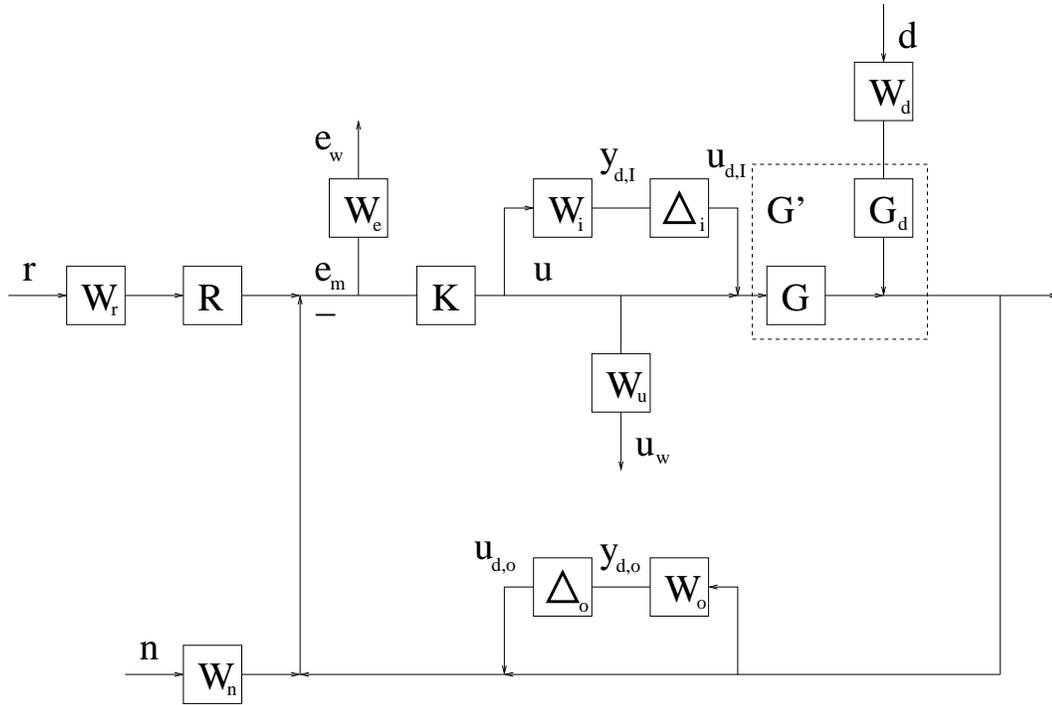
Figure 7.13: Block diagram for  $\mu$ -analysis
