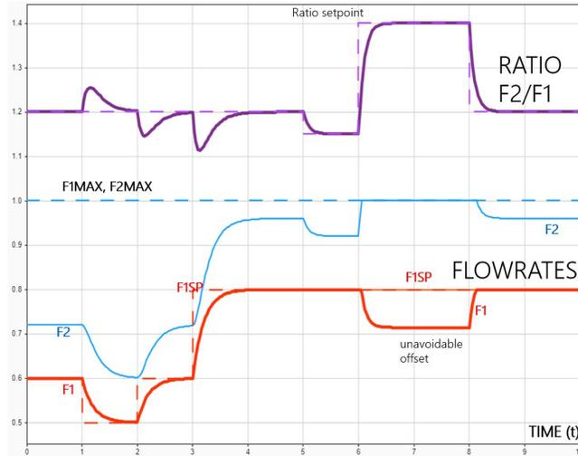
Figure 10: Simulation of modified dual ratio SRC scheme in Figure 9.
