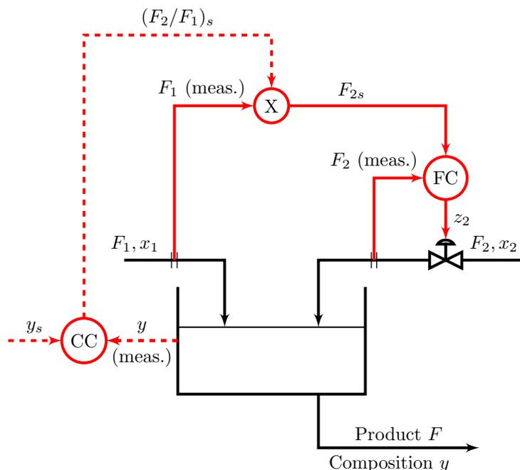
Figure 1: Recommended ratio control scheme for mixing process. The ratio setpoint  $(F_2/F_1)_s$  is set by an outer composition controller (CC). The signals denoted (meas.) need to be measured or estimated.
