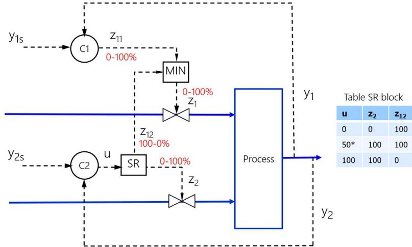
Figure 15: General split-range control for MV-MV switching combined with override MIN-selector for CV-CV switching (for case where control of  $y_2$  has higher priority than control of  $y_1$ ). Controller C1 has anti-windup but not the split-range controller C2. (\*The split value of 50% in the table may be changed to adjust the effective controller gain).
