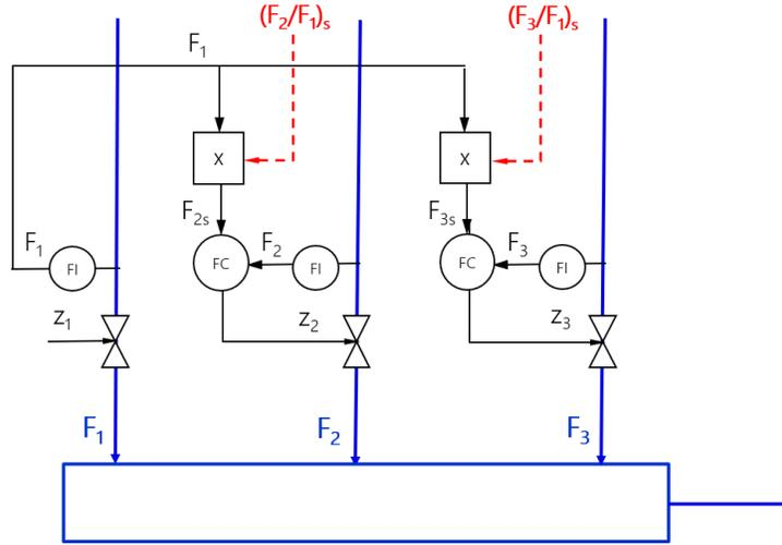
Figure 4: Ratio control for process with three independent extensive variables (flows) where  $F_1$  is a disturbance and  $F_2$  and  $F_3$  are manipulated. Here, we need to set two ratios, which in this case are selected as  $F_2/F_1$  and  $F_3/F_1$ .
