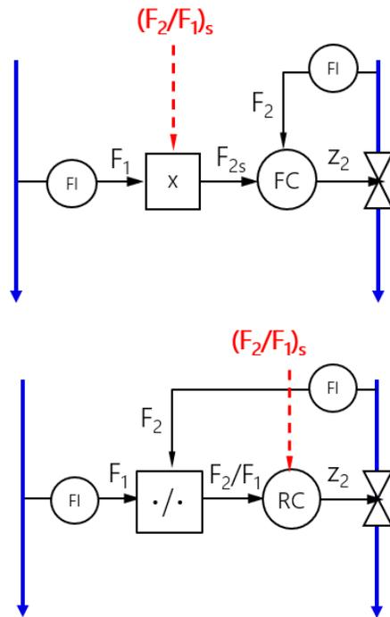
Figure 3: Two alternatives schemes for implementing ratio control (Buckley (1964), Figures 17.5 and 17.7) (Shinskey, 1967) (Luyben, 1973).
