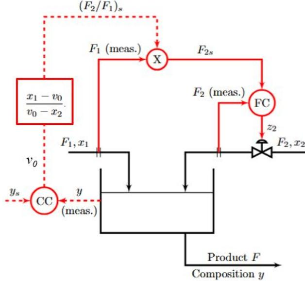
Figure 14: Improved ratio control scheme for mixing process using transformed input  $v_0$ . The feed mass fractions  $x_1$  and  $x_2$  that enter the computation block, need to be measured or estimated.
