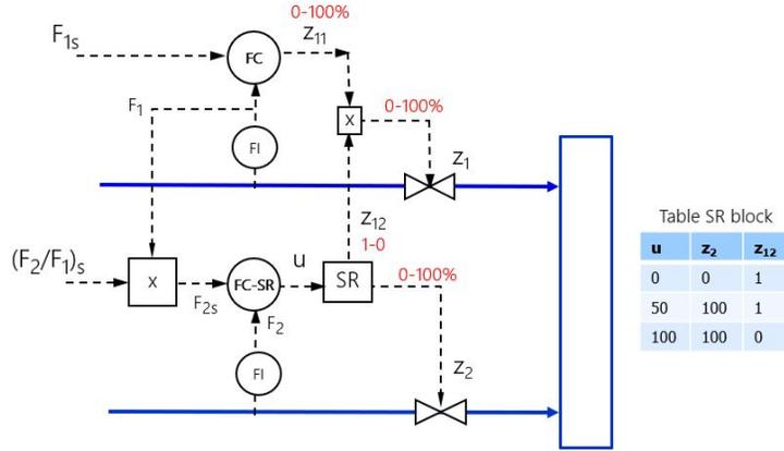
Figure 9: Modified split-range control (SRC) scheme for “dual” ratio control where the MIN-selector in Figure 7 is replaced by multiplication to avoid the limbo effect.
