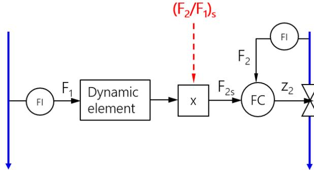
Figure 6: Ratio control with dynamic compensation. The dynamic element has no effect at steady state.
