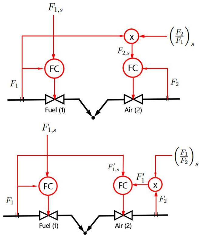
Figure 11: Conventional ratio control implementations for combustion. The two schemes are equivalent for practical purposes. The second scheme with the inverse ratio is shown as an intermediate step to the cross-limiting scheme in Figure 12.
