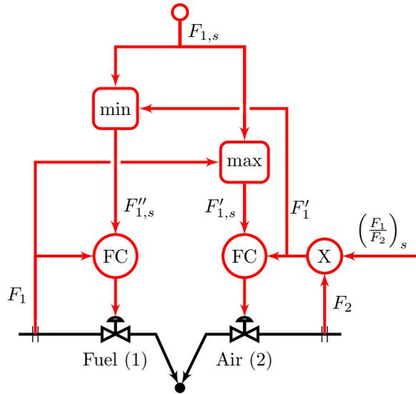
Figure 12: Cross-limiting ratio control for combustion where air (2) should always be in excess of fuel (1) (Smith & Corripio, 1997; Wade, 2004).
