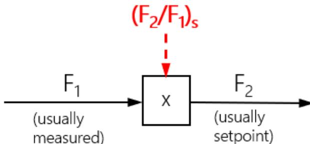
Figure 2: Multiplication element to compute  $F_2 = (F_2/F_1)_s \cdot F_1$  where  $F_1$  is the basis and  $(F_2/F_1)_s$  is the desired ratio (setpoint).
