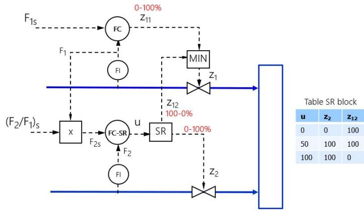
Figure 7: "Dual" ratio control using split-range control (SRC)
