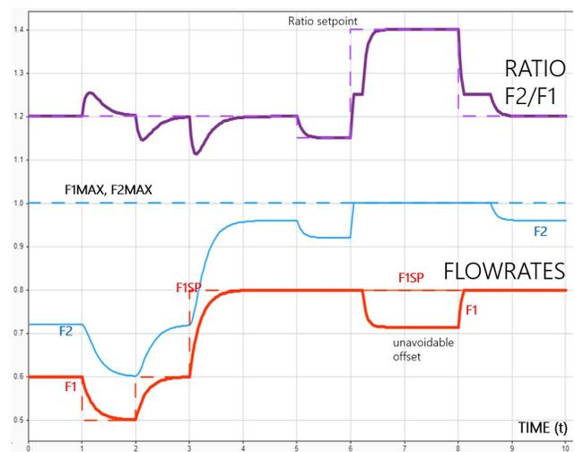
Figure 8: Simulation of dual ratio SRC scheme in Figure 7. The limbo-effect, caused by a delay from the MIN-selector, is seen for the ratio at times 6 and 8.
