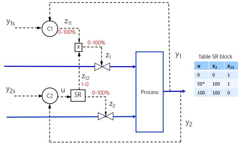
Figure 16: Avoiding limbo-effect with split-range control by replacing the MIN-selector in Figure 15 by a multiplication element. Controller C1 has anti-windup but not the split-range controller C2. (\*The split value of 50% in the table may be changed to adjust the effective controller gain for C2).
