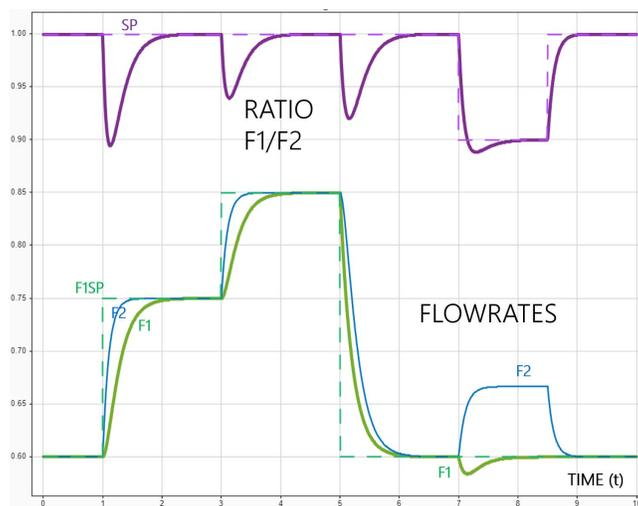
Figure 13: Simulation of the cross-limiting ratio control scheme in Figure 12.
