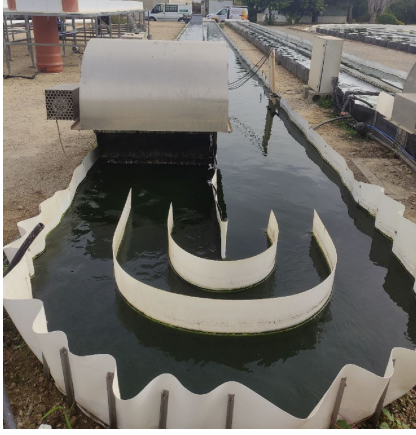
Fig. 1. Raceway reactor subject of this work.
