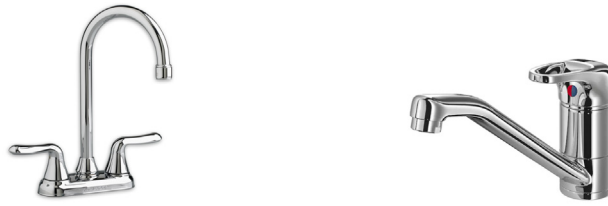
(a) Traditional design with two separate handles ( u_1 = F_1, u_2 = F_2 ) (b) Modern one-handle design where decoupling is achieved by the physical design ( v_1 = F_1 + F_2 and v_2 = \frac{F_1}{F_2} ).
