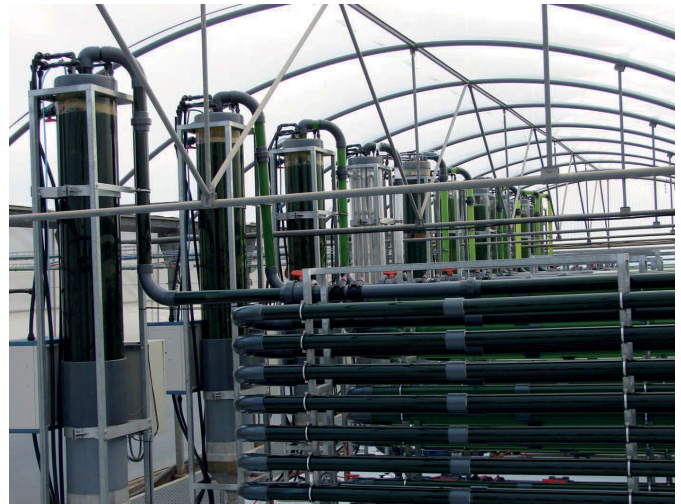
Fig. 1. Real view of a tubular photobioreactor at the Las Palmerillas experimental station, Almería (Spain).
