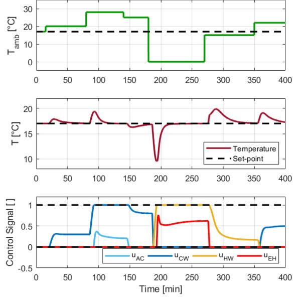
Figure 5. GSRC results. Top: Temperature profile for the scenario. Middle: Internal temperature. Bottom: manipulated variables for each actuator.
