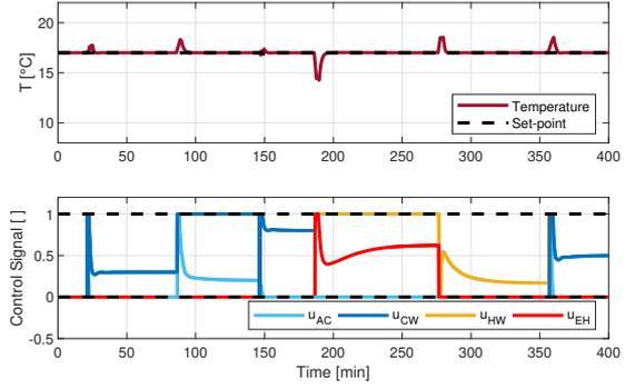
Figure 6. SRGPC results for the same disturbance sequence. Top: Internal temperature. Bottom: manipulated variables for each actuator.
