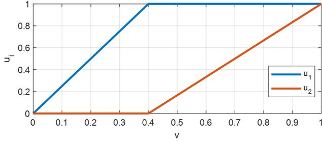
Figure 2. Split-range profile input usage regarding the controller output  $v$ .
