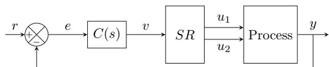
Figure 1. Split range control strategy for a Two-Input Single-Output system.
