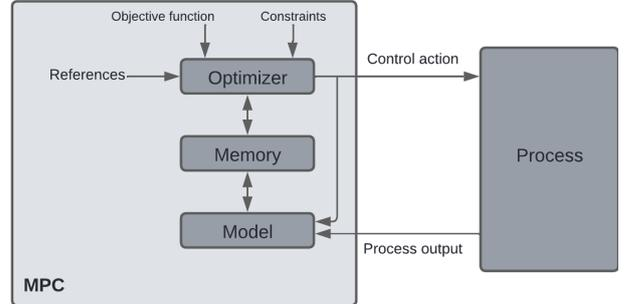
Figure 4. Basic MPC structure.
