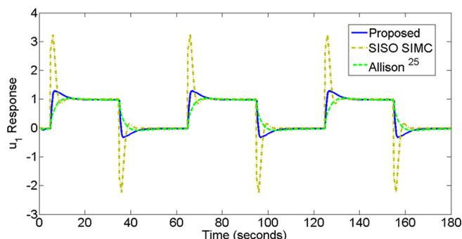
**Figure 6.** Nominal manipulated variable response in  $u_1$  for Example 1.
