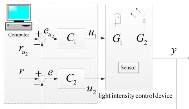
Figure 20. Light intensity control experiment schematic.
