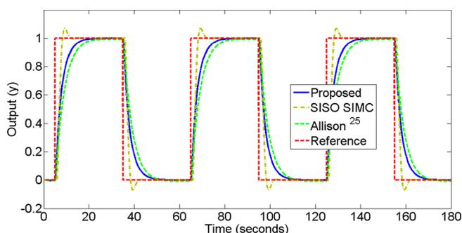
**Figure 4.** Nominal output response in  $y$  to unit step square wave reference for Example 1.
