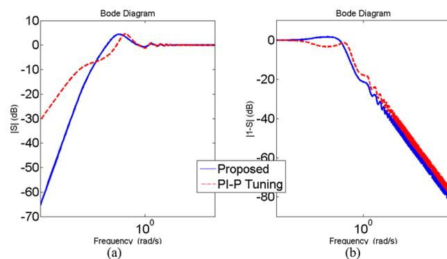
Figure 15. (a) Sensitivity function  $S$ . (b) Complementary sensitivity function  $T$ .
