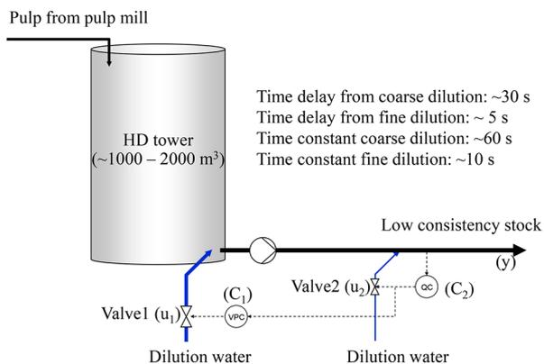
Figure 11. Paper pulp consistency control schematic.
