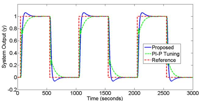
Figure 12. Uncertain output response in  $y$  to unit step square wave reference for Example 2.
