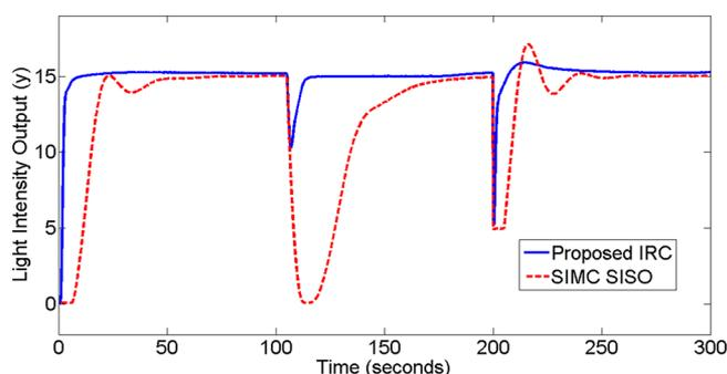
Figure 21. Measurement sensor output for the light intensity control experiment.
