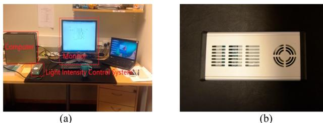
Figure 19. (a) Light intensity control experiment apparatus. (b) Light intensity control device.
