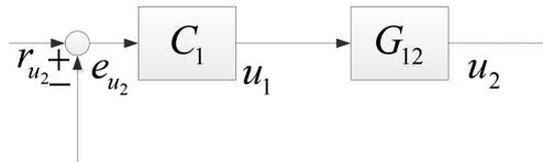
Figure 3. Diagram of the equivalent closed-loop for  $G_{12}$ .
