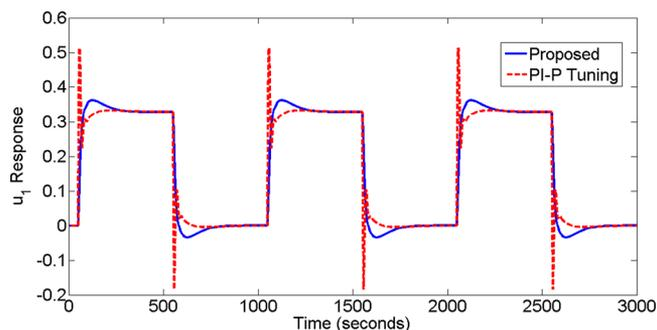
Figure 14. Uncertain manipulated variable response in  $u_1$  for Example 2.
