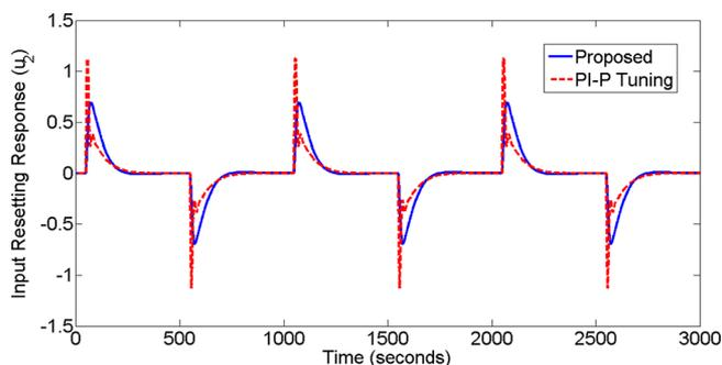
Figure 13. Uncertain input resetting response in  $u_2$  for Example 2.
