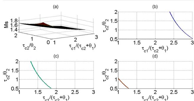
Figure 10. (a) Surface of  $M_s$  value to parameters  $\tau_{c1}$  and  $\tau_{c2}$ . (b) Region of the combination of  $\tau_{c1}$  and  $\tau_{c2}$  with  $M_s = 1.4$ . (c)  $M_s = 1.6$ . (d)  $M_s = 1.8$ .
