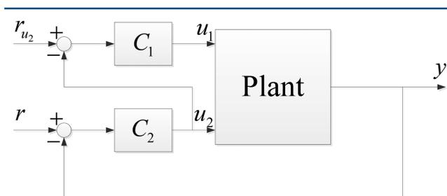
Figure 1. General cascade implement of input resetting control.
