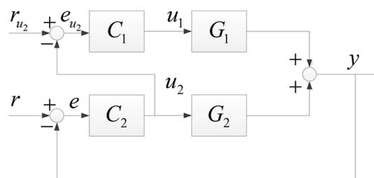
Figure 2. Two inputs and single output cascade implement of input resetting control.
