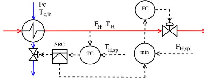
Figure 3: Split range control structure for cooler.
