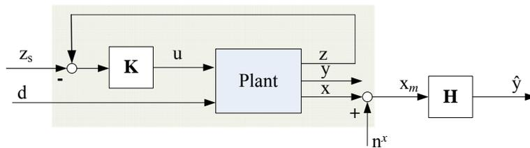
(c) S3: Monitoring case where  $u$  is used to control the secondary variable  $z$
