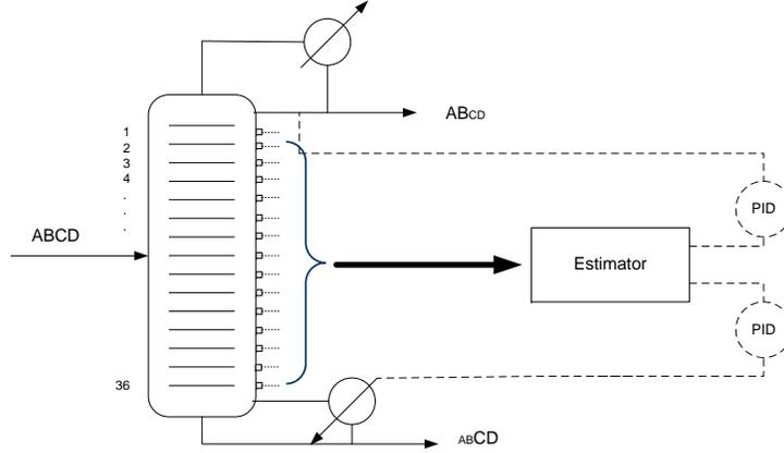
Figure 5: Schematic of the distillation process with estimator
