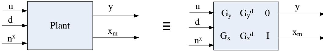
Figure 2: Block diagram for the linearized plant
