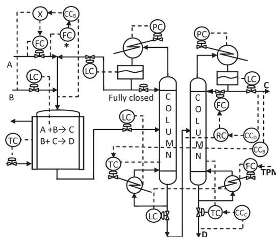
Figure 7. Regulatory control structure with  $Q_{reb2}$  as TPM. The asterisk (\*) indicates FC adjusting  $CC_B$  set point to get desired  $F_A$  processing rate.
