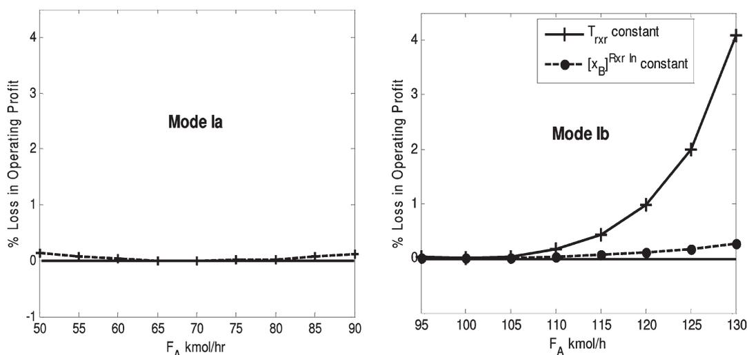
**Figure 4.** Percentage loss in profit for process operation at constant  $T_{rxr}$  and/or constant  $[x_B]^{RrxrIn}$ . (left) Mode Ia: loss with both  $T_{rxr}$  and  $[x_B]^{RrxrIn}$  constant. (right) Mode Ib: loss with either  $T_{rxr}$  constant or  $[x_B]^{RrxrIn}$  constant.
