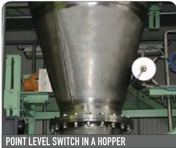
POINT LEVEL SWITCH IN A HOPPER Figure 4. A narrowly collimated conical beam is aimed across the vessel at the point detector.
