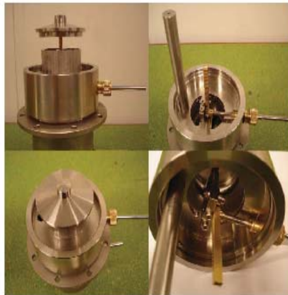
From top left: Valve in fully open position Top right: Rack and pinion arrangement.
