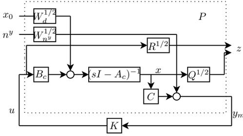
Fig. 2. Interconnection structure for closed-loop optimization of  $K$ .
