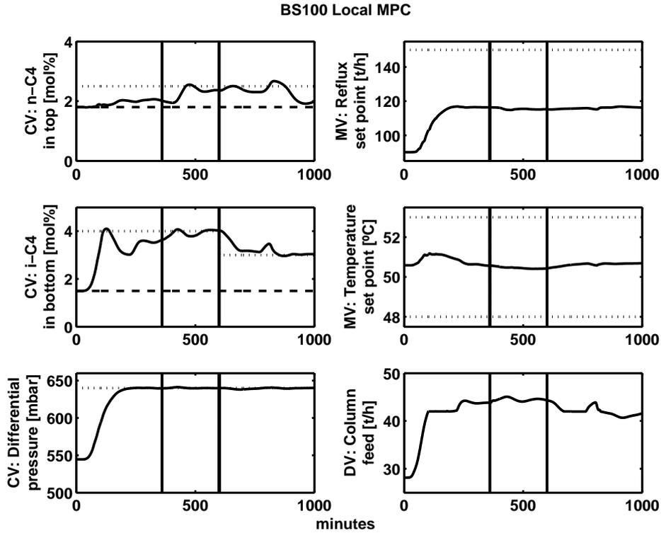
Fig. 6. CVs, MVs and DV to the butane splitter in T-100. Vertical lines indicate new case.
