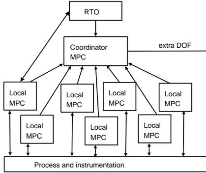
Fig. 1. The control hierarchy with the coordinator MPC
