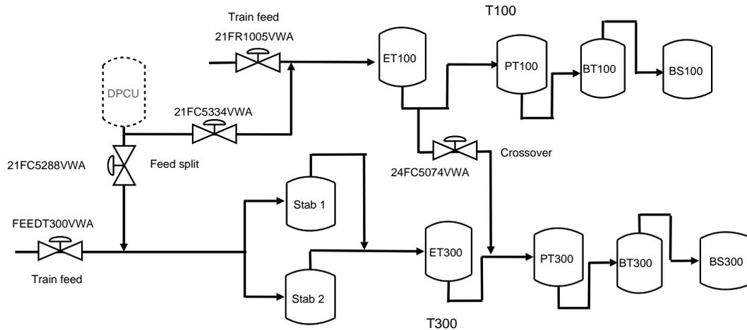
Fig. 3. The simulated parts of the Kårstø plant
