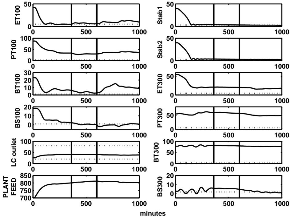
Fig. 4. CVs in the coordinator MPC, remaining feed capacity and plant feed in t/h, LC outlet in %. Vertical lines indicate new case.
