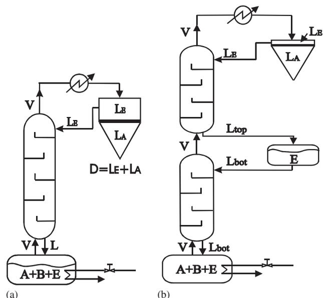
Fig. 1. Heteroazeotropic batch distillation in (a) conventional rectifier column and (b) multivessel column.
