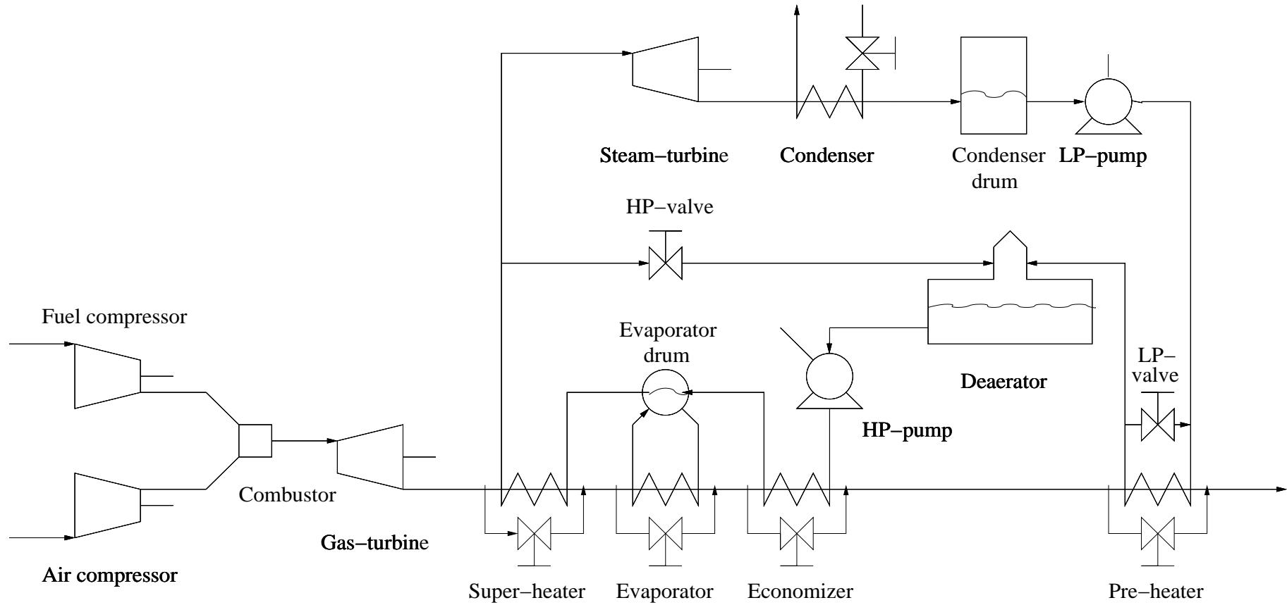
DOF: 13-2(levels without steady-state effect)-1(deaerator pressure)-2(turbine speeds)=8
