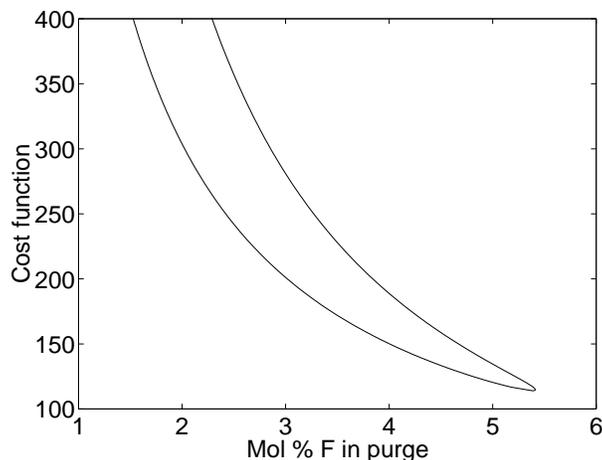
Figure 5: Unfavorable shape of cost function with % F (byproduct) in purge as controlled variable. Shown for case with constant reactor temperature and C in purge.
