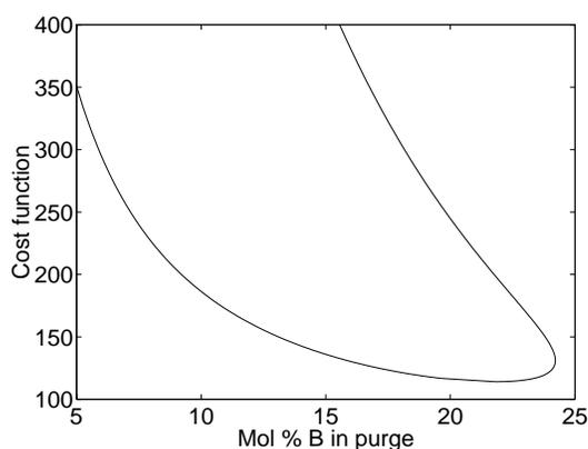
Figure 9: Typical unfavorable shape of cost function with B (inert) in purge as controlled variable (shown for case with constant reactor temperature and C in purge).
