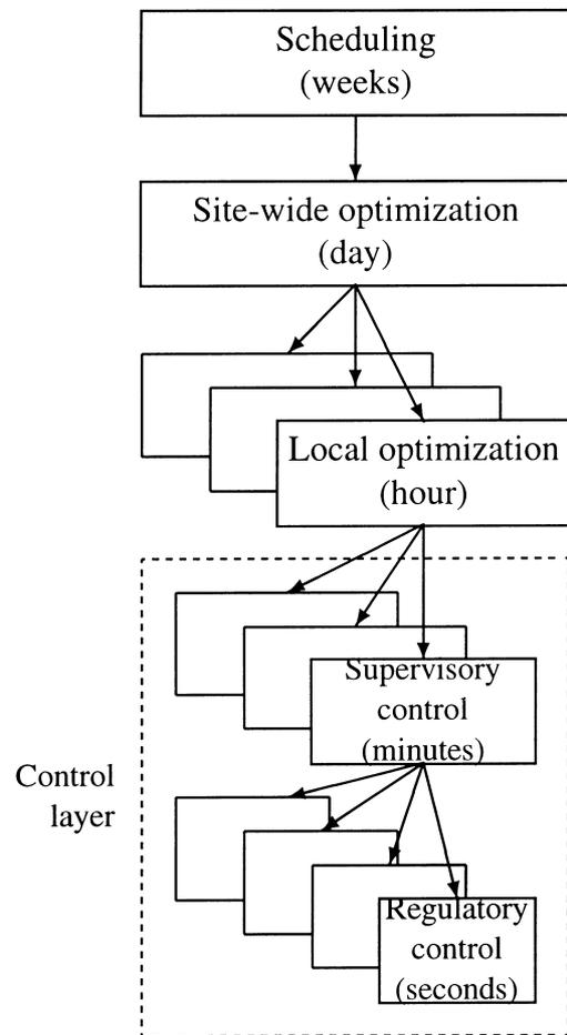
Fig. 1. Typical control hierarchy in a chemical plant.
