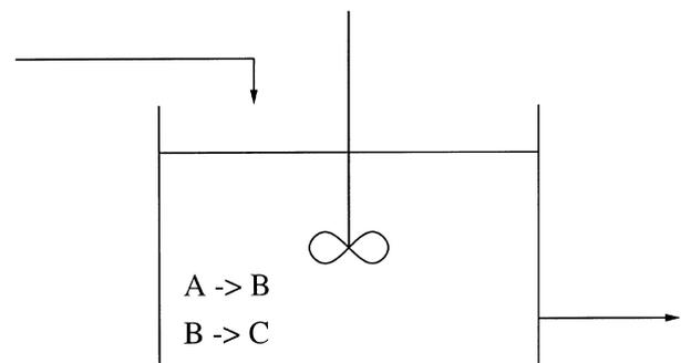
Fig. 6. Reactor example where the objective is to maximize fraction of B,  $x_B$ .
