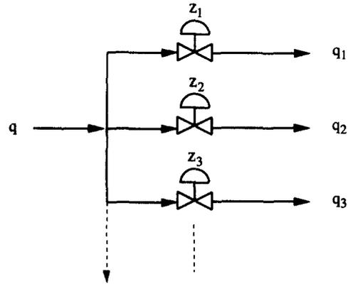
FIG. 2. Splitting into parallel streams (Example 1).
