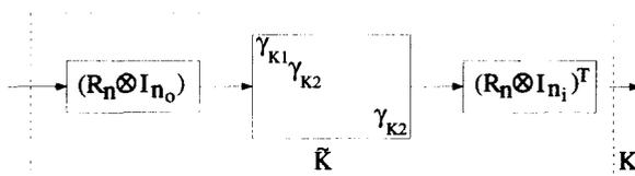
FIG. 6. Realization of a full block parallel controller  $K$ .
