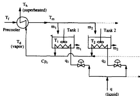
FIG. 3. Cooling system for parallel reactors (Example 2).
