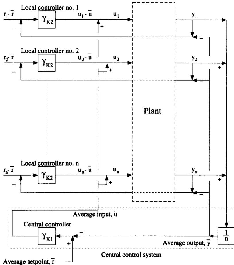
FIG. 9. Distributed implementation of a full block parallel controller  $K$ .
