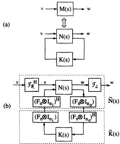
FIG. 4. (a) Expressing  $M(s)$  as a linear fractional transformation of the controller  $K(s)$ . (b) Pre and postmultiplication of  $M(s)$  by unitary matrices.
