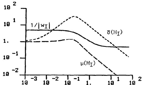
Fig. 3. Robust stability for the distillation column with diagonal input uncertainty is guaranteed since  $\mu(H_I) \leq 1/|w_I| \forall \omega$ . The use of unstructured uncertainty and  $\bar{\sigma}(H_I)$  is conservative, and would require the system to be detuned to guarantee robust stability.
