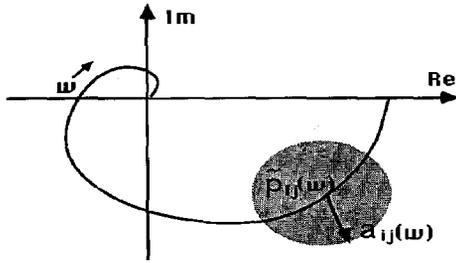
Fig. 8. Additive element uncertainty:  $|p_{ij} - \tilde{p}_{ij}| < a_{ij}(\omega)$ . The disc represents the set of possible  $p_{ij}(j\omega)$  at a given frequency.
