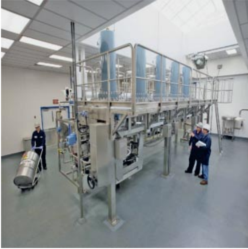
Figure 19. Simulated moving bed chromatographic process for API purification (courtesy of AMPAC Fine Chemicals, Rancho Cordova, CA, USA)
