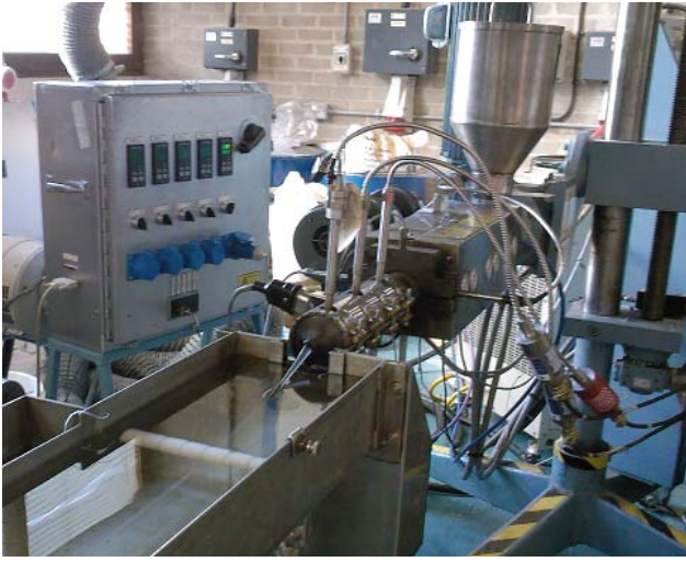
Fig. 2: The laboratory extruder with a in-line-rheometer die
