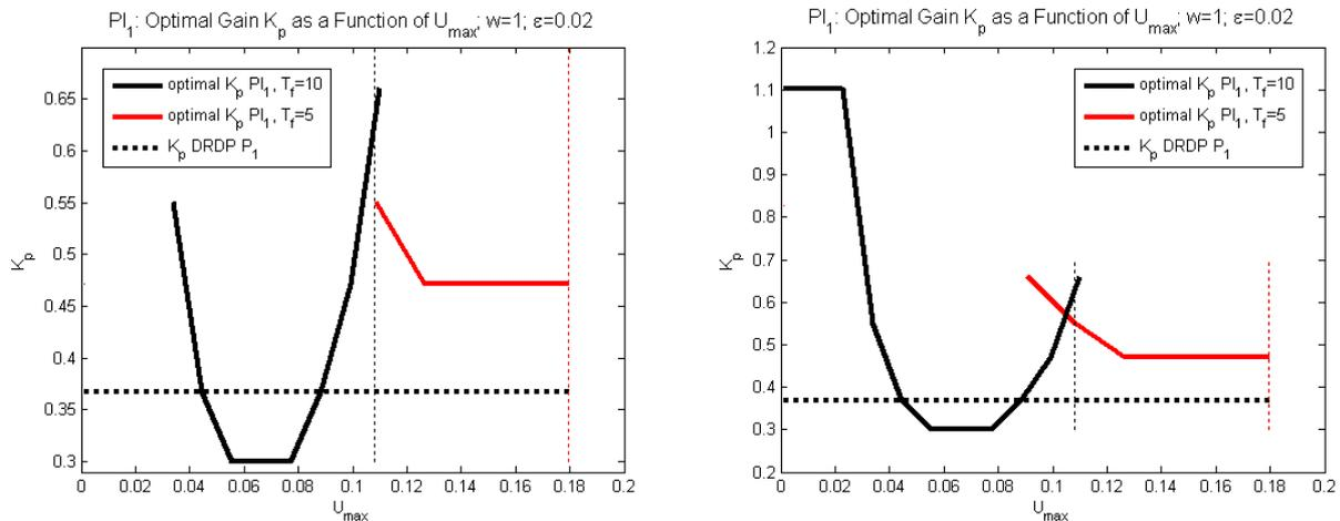
Figure 10 Influence of the saturation level  $U_m$  on the optimal gain of the  $PI_1$ -DOB controller for two different values of the DOB filter time constant  $T_f$  and  $\varepsilon = \varepsilon_y = \varepsilon_u = 0.02$  (left relative precision for  $u$ -1P, right absolute precision)
