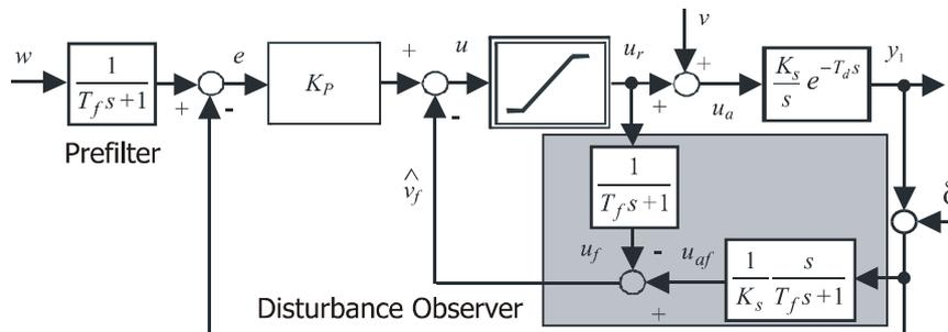
Figure 4 Disturbance observer based  $PI_1$  controller with inverse dominant plant dynamics and possible prefilter
