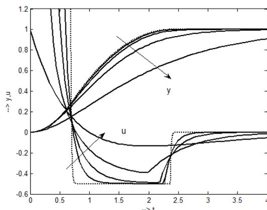
Figure 2 Output and control signal transients of double integrator plant by constrained PAC  $U_{max}=1.2$  and  $U_{min}=-0.5$  for the double real pole values -8, -4, -2 and -1 – arrows indicate pole shifting to zero (i.e. slowing down transients); dotted – MTC transients
