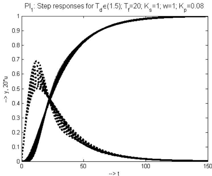
Figure 7 Example of  $y_1$ -MO &  $u$ -1P step responses corresponding to the ULS from Fig. 6 with the lowest mean IAE value;  $T_f = 20; T_d \in (1,5); K_s = 1$ ;
