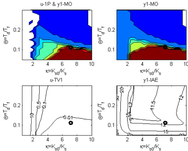
Figure 5 Example of the 2D performance portrait with the point corresponding to  $y_1$ -MO &  $u$ -1P step response with the lowest IAE value;
