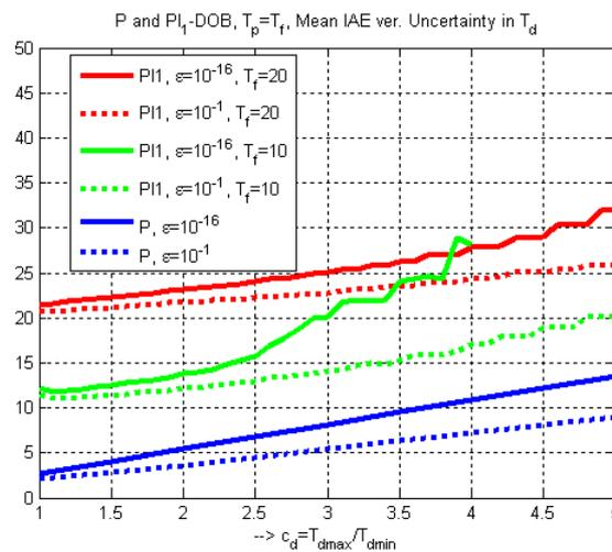
Figure 8 Influence of the uncertainty in  $T_d$  characterized by  $c_d = T_{d \max} / T_{d \min}$  on the mean IAE values of the P and of the PI<sub>1</sub>-DOB with  $T_f = 20$  and  $T_f = 10$
