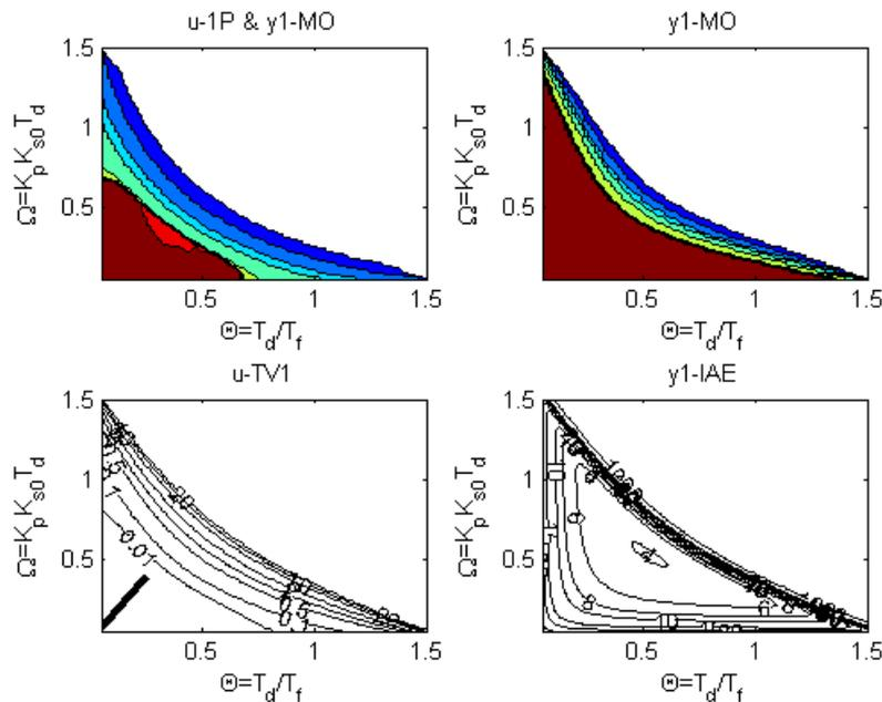
Figure 6 Example of the 2D performance portrait with the ULS corresponding to  $y_1$ -MO &  $u$ -1P step response
