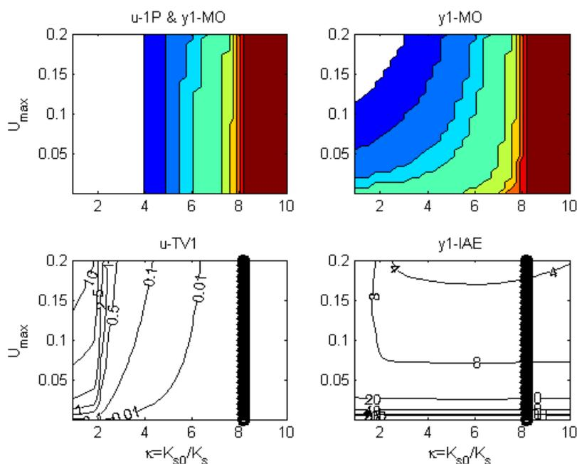
Figure 9a Influence of the saturation level  $U_m$  on the optimal working point  $\kappa$  of the P controller;
