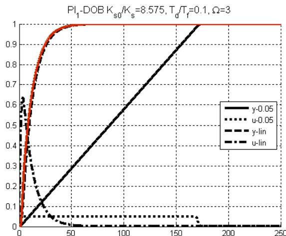
Figure 11 Step responses corresponding to the optimal tuning identified for the saturation level  $U_m = 0.05$  and used then also for the unconstrained case (black) and the output step response corresponding to the optimal gain for the unconstrained case (red);  $T_f = 10$ ;  $T_d = 1$ ;  $K_s = 1$ ;  $\Omega = 3$
