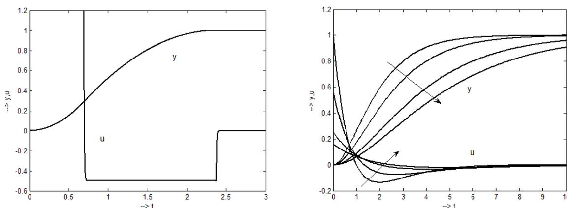
Figure 1 Output and control signal transients of the double integrator plant: left - for the relay MTC with control signal constrained by  $U_{max}=1.2$  and  $U_{min}=-0.5$ ; right – for the linear PAC with the double real pole values -1, -0.75, -0.5 and -0.4 - arrows indicate pole shifting to zero (i.e. slowing down transients)
