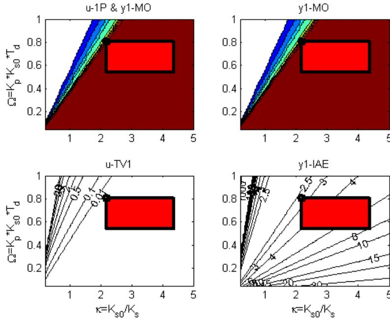
Figure 3 Performance portrait of the linear loop with the P-controller and IPTD plant; optimal point corresponds to the whole line (16); Uncertainty Box (17) corresponding to plan parameters (11) (red)
