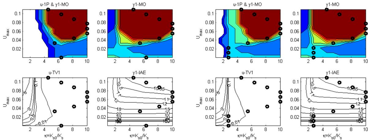
Figure 9b Influence of the saturation level  $U_m$  on the optimal working point  $\kappa$  of the  $PI_1$ -DOB controller for  $\varepsilon = \varepsilon_y = \varepsilon_u = 0.02$  for the DOB filter time constant  $T_f = 10$ ;  $\Omega = 3$ ;  $T_d = 1$ ;  $K_s = 1$ ;  $\varepsilon = \{0.1, 0.05, 0.02, 0.01, 10^{-3}, 10^{-4}, 10^{-5}, 10^{-6}, 10^{-16}\}$  (from blue to brown, left relative precision for  $u$ -1P, right absolute precision)
