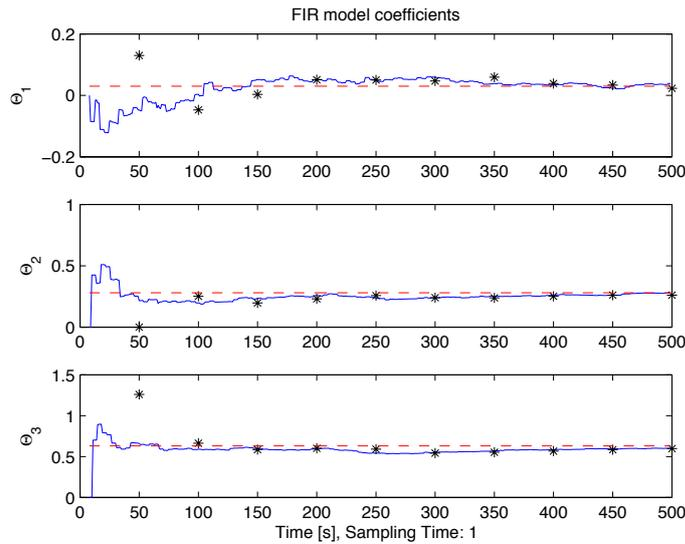
FIGURE 2. FIR parameters: RLS estimates (solid line), ‘real’ values (dashed line), MPC model parameter (stars).
