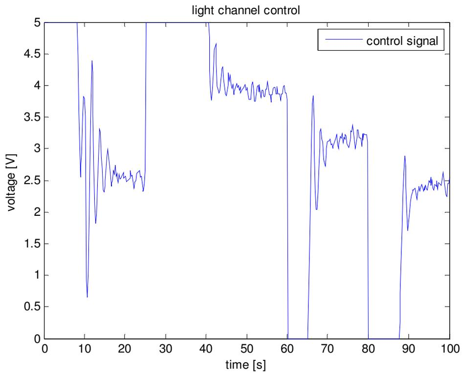
Figure 8b: Closed-loop - several setpoint changes;  $K_{s0} = \text{mean}\{K_s\}$
