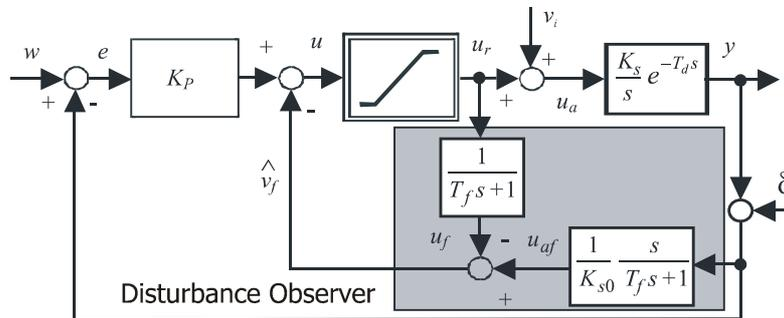
Figure 6: PI<sub>1</sub>-controller
