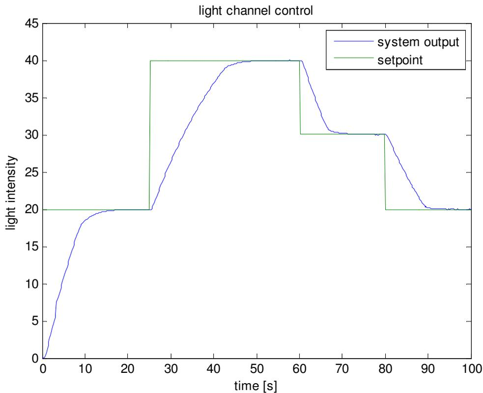
Figure 7a: Closed-loop - several setpoint changes;  $K_{s0} = \max\{K_s\}; T_{d0} = \max\{T_d\}$
