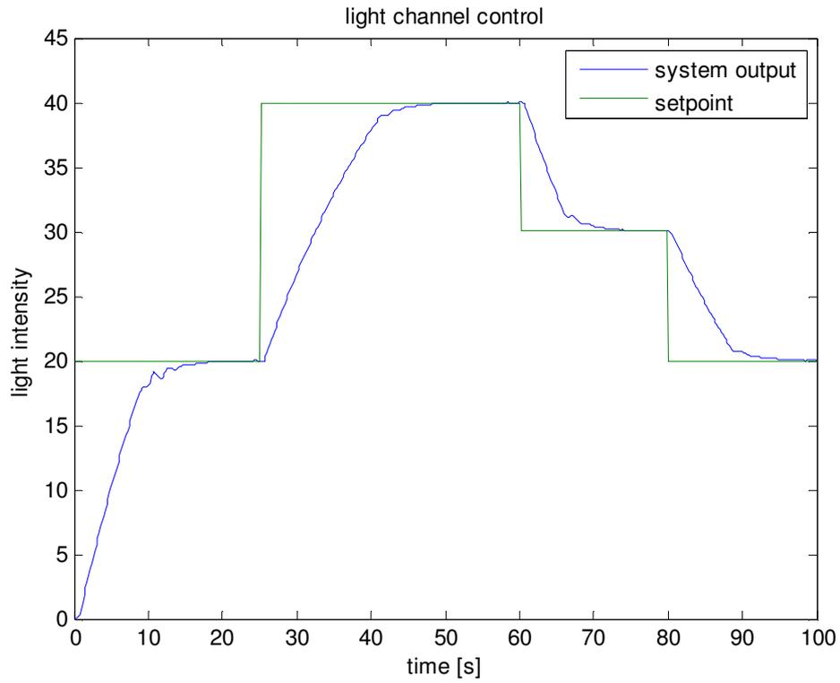
Figure 8a: Closed-loop - several setpoint changes  $K_{s0} = \text{mean}\{K_s\}$
