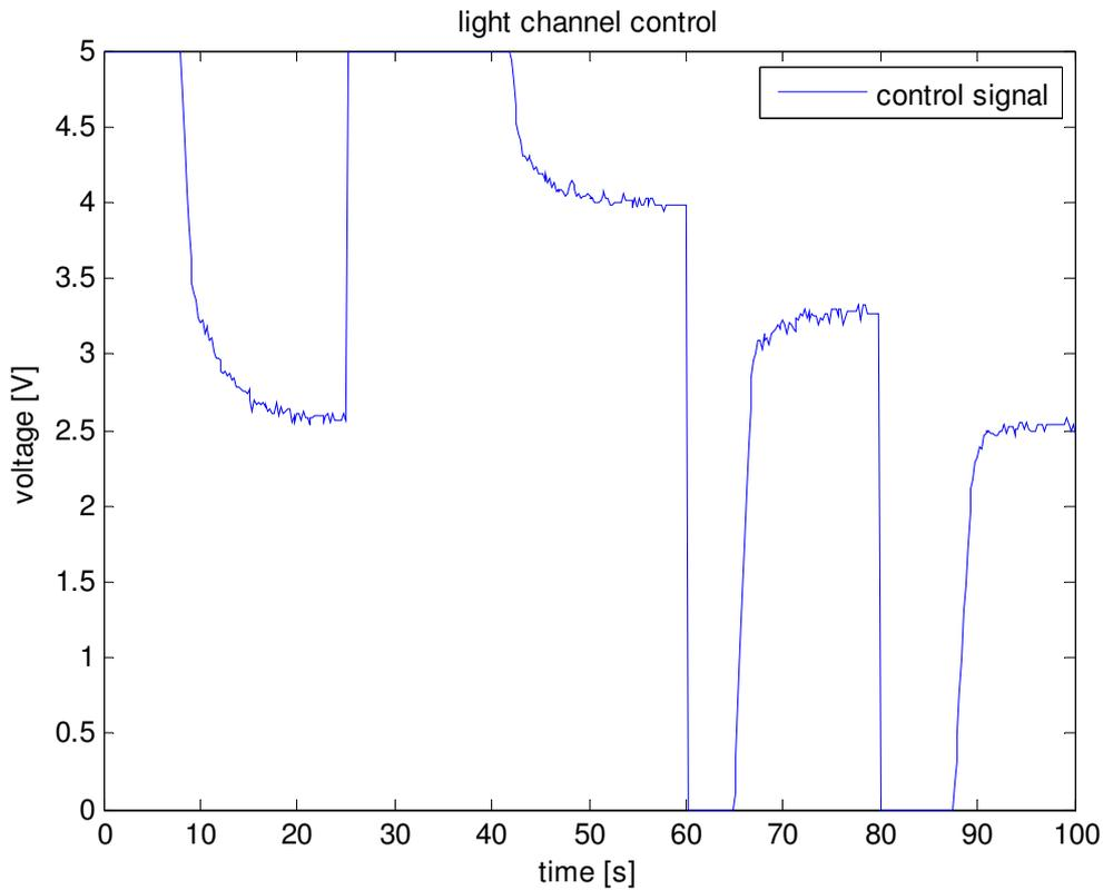
Figure 7b: Closed-loop - several setpoint changes;  $K_{s0} = \max\{K_s\}; T_{d0} = \max\{T_d\}$
