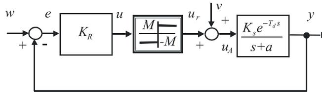
Figure 2: Relay identification with nonsymmetrical plant input
