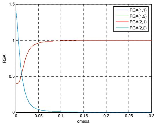
Figure 2a: RGA for minimum phase case ( $\gamma_1=0.6, \gamma_2=0.8$ )
