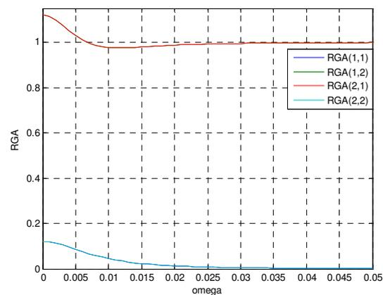
Figure 2b: RGA for non-minimum phase case ( $\gamma_1=0.2, \gamma_2=0.3$ )
